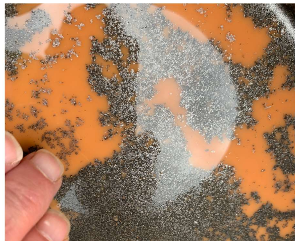
Figures 6 & 7: Very coarse-flake graphite in +600µm sample fraction (L), graphite floating on soaking drill sample (R)
