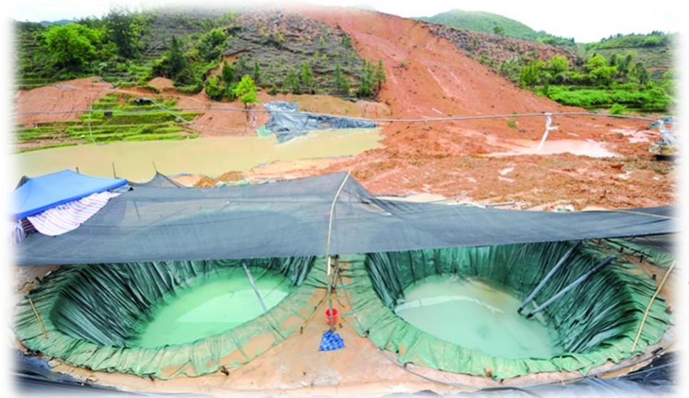
Southern China in situ leach mining operation
