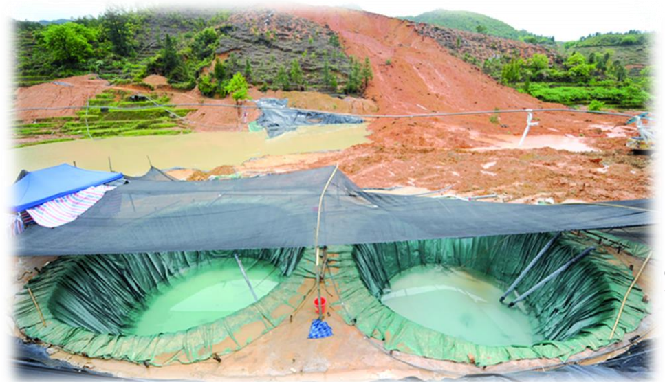
Southern China in situ leach mining operation
