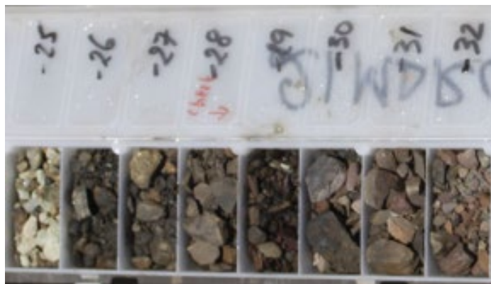
Image 5 / RC drill chips: 21MDRC040 24-32m (8m @ 0.84 % Cu & 960 ppm Co malachite & chalcocite mineralisation)
