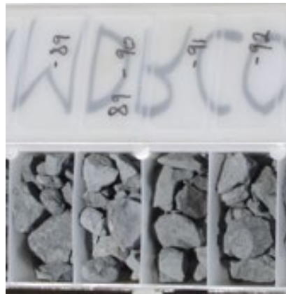
Image 4 / RC drill chips: 21MDRC033 88-92m (4m @ 1.27 % Cu & 212 ppm Co sulphide chalcopyrite and chalcocite mineralisation)
