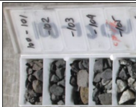
Image 2 / RC drill chips: 21MDRC027, 86-106m (20m @ 1.60 % Cu & 794 ppm Co, transitional to sulphide chalcopyrite and chalcocite mineralisation)
