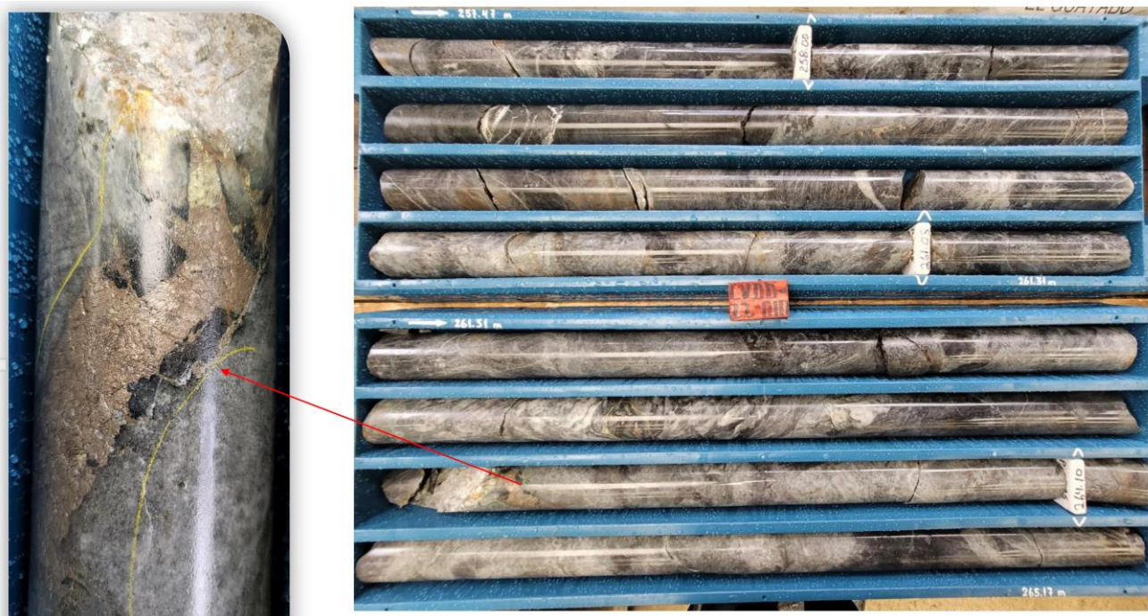
Photo - CVDD-22-10 (close up 263m): 161-363m logged as Intrusive Breccia containing sulphides (Po3%, Py 0.5%, Cpy 0.5%) in clasts and 2% sulphides in matrix
