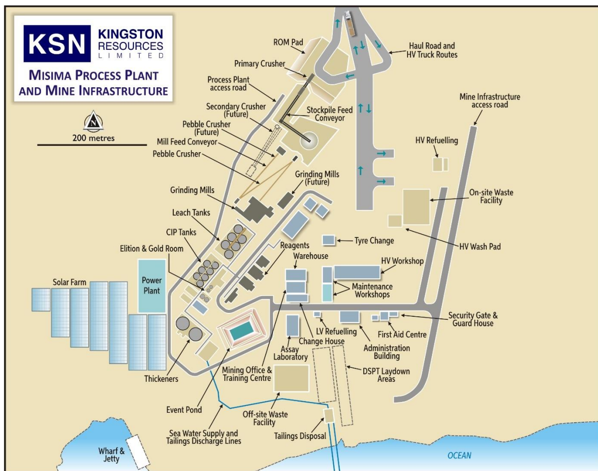
Figure 2: Misima Gold Project plant layout
