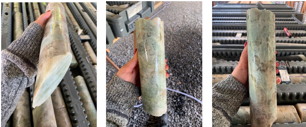
Figure 3: Drill core from SADD017 showing large light-green fresh spodumene crystals
