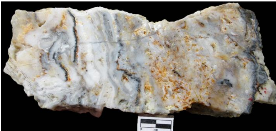
Figure 1: Sample of quartz vein from the Rek Rinti vein system showing black, sulphide rich ginguro bands. Sample assay of 38.14 g/t Au, 581 g/t Ag.
