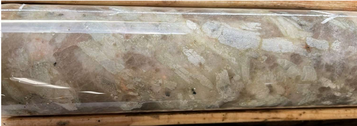
Figure 3: A close-up image of MF22-80 (Hole 21) showing large silvery-white coloured spodumene crystals
