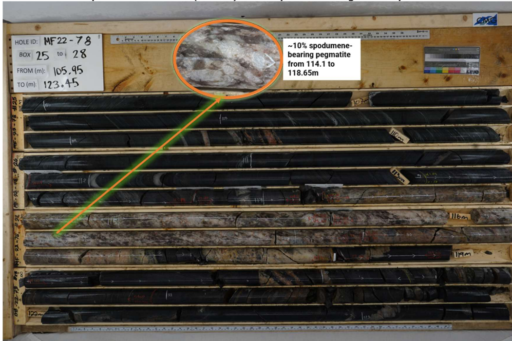
Figure 6: White pegmatite hosts approximately 10% of fine to medium-white-grey, spodumene crystals intersected from 114.1 to 118.65 metres depth in Hole MF22-78 (Hole 19). Close-ups illustrate significant spodumene mineralisation.
