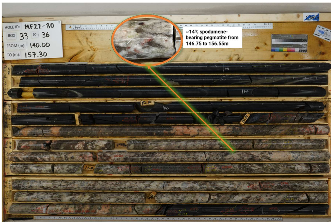
Figure 4: White pegmatite hosts approximately 14% of fine to medium, silver-white, spodumene crystals intersected from 146.75 to 156.55 metres depth in Hole MF22-80 (Hole 21). Close-ups illustrate significant spodumene mineralisation.
