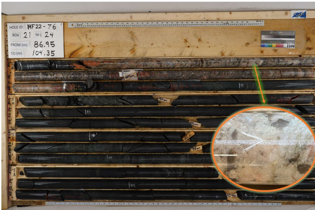
Figure 8: White to grey pegmatite hosts approximately <5% of fine to large, white grey, spodumene crystals intersected from 87.25 to 90.2 metres depth in Hole MF22-76 (Hole 17). Close-ups illustrate significant spodumene mineralisation
