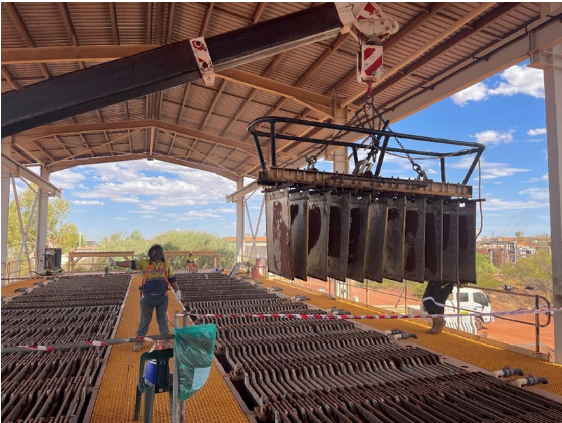
Image 5 / EW - Removal of Cathodes
