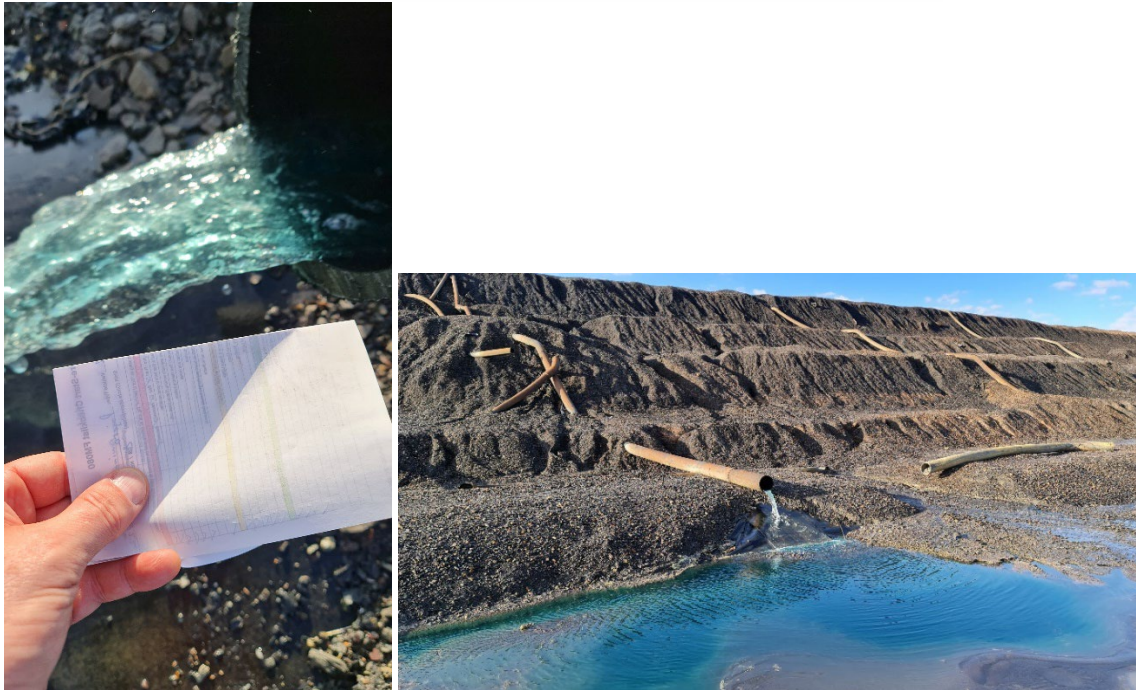
Image 15 / Copper rich solution flowing out of the heaps following recent rainfall at Nifty, for future solution inventory
