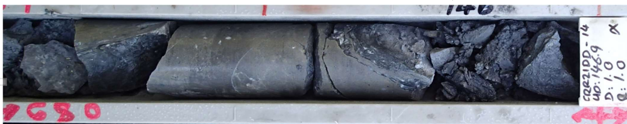
Figure 2: CRR21DD_014, detail from above Figure 1 of Sample (42)680 (146.51-146.90m downhole) exhibiting extensive massive sulphide – sample assayed 31.30% Zn, 18.30% Pb, 0.60% Cu, 59.30g/t Ag (NQ core, 50mm diameter)
