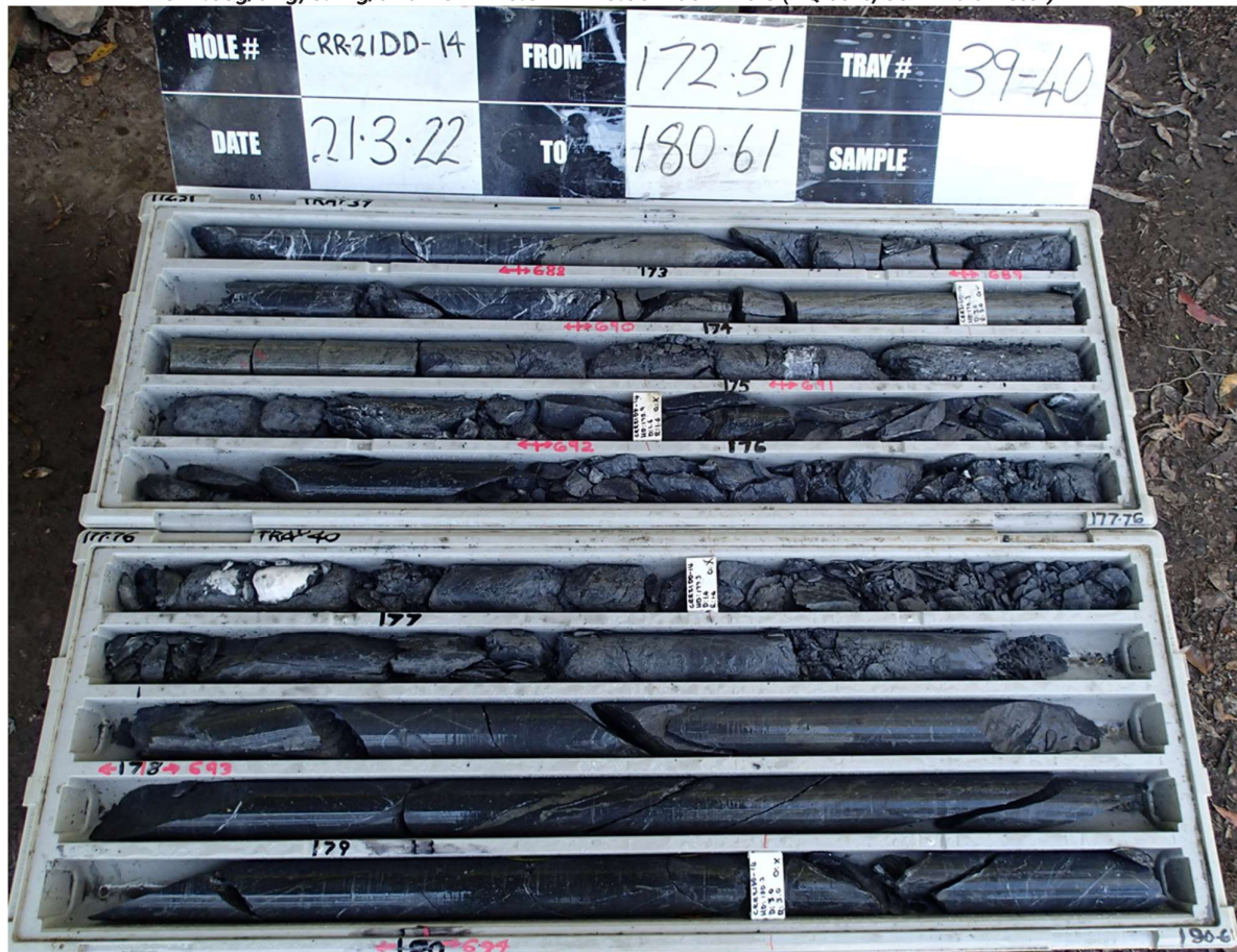
Figure 4: CRR21DD_014, detail from above Figure 3 of Sample (42)690 (173.84-175.06m downhole) exhibiting extensive banded, massive sulphide – sample assayed 25.40% Zn, 15.50% Pb, 3.46% Cu, 394.00g/t Ag, 0.44g/t Au (NQ core, 50mm diameter)
