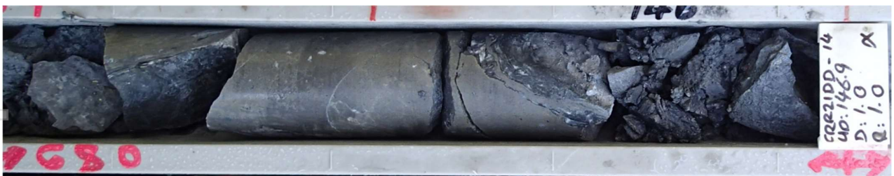
Figure 2: CRR21DD_014, detail from above Figure 1 of Sample (42)680 (146.51-146.90m downhole) exhibiting extensive massive sulphide – sample assayed 31.30% Zn, 18.30% Pb, 0.60% Cu, 59.30g/t Ag (NQ core, 50mm diameter)
