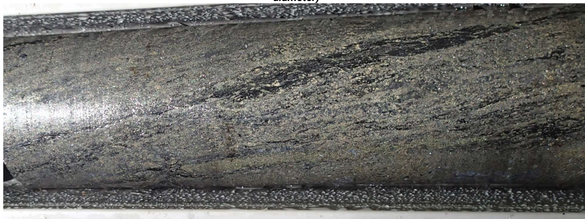
Figure 4: CRR21DD_014, detail from above Figure 3 of Sample (42)690 (173.84-175.06m downhole) exhibiting extensive banded, massive sulphide – sample assayed 25.40% Zn, 15.50% Pb, 3.46% Cu, 394.00g/t Ag, 0.44g/t Au (NQ core, 50mm diameter)
