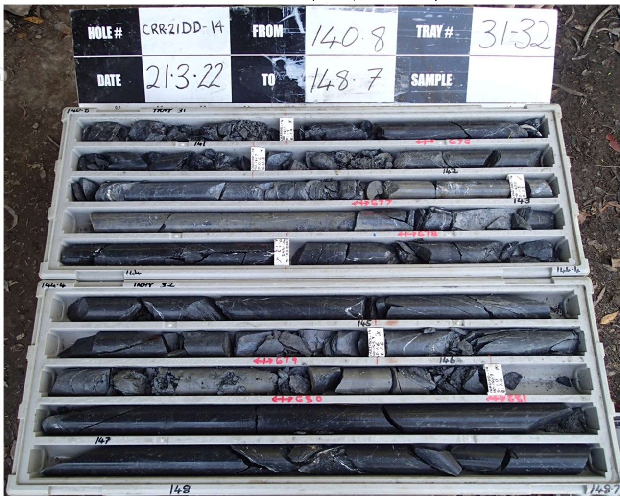
Figure 2: CRR21DD_014, detail from above Figure 1 of Sample (42)680 (146.51-146.90m downhole) exhibiting extensive massive sulphide – sample assayed 31.30% Zn, 18.30% Pb, 0.60% Cu, 59.30g/t Ag (NQ core, 50mm diameter)
