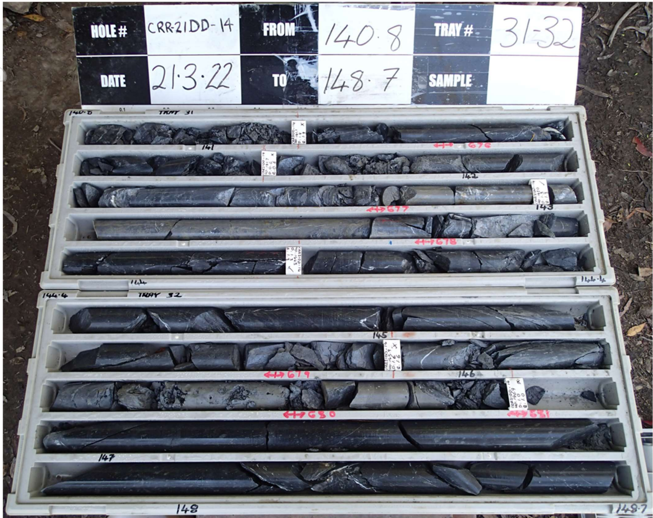
Figure 2: CRR21DD_014, detail from above Figure 1 of Sample (42)680 (146.51-146.90m downhole) exhibiting extensive massive sulphide – sample assayed 31.30% Zn, 18.30% Pb, 0.60% Cu, 59.30g/t Ag (NQ core, 50mm diameter)
