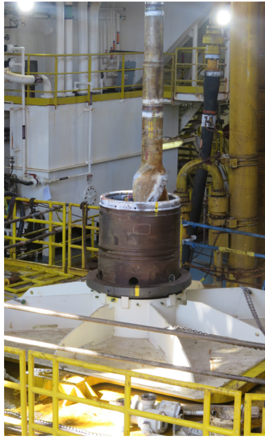
Downhole drilling assembly and installation within the well head housing on the mudmat
