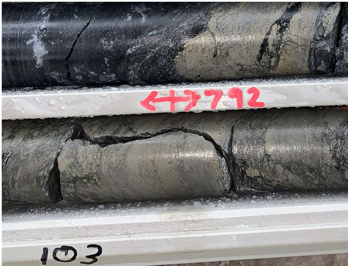
Figure 7: CRR21DD_04, Portion of sample 384796 (104.40-104.68m downhole) exhibiting extensive massive sulphide with abundant brassy yellow chalcopyrites (copper sulphide mineral) – sample assayed 15.4% Zn, 0.58% Pb, 13.30% Cu, 71.9g/t Ag and 0.17g/t Au, part of the longer downhole interval of 6.91m @ 9.41% Zn, 2.45% Pb, 1.56% Cu, 34.6g/t Ag, 0.23g/t Au from 98.04-104.95m downhole (NQ core, 50mm diameter)
