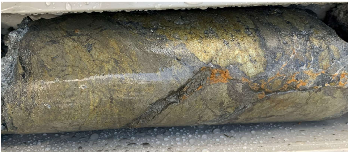
Figure 7: CRR21DD_04, Portion of sample 384796 (104.40-104.68m downhole) exhibiting extensive massive sulphide with abundant brassy yellow chalcopyrites (copper sulphide mineral) – sample assayed 15.4% Zn, 0.58% Pb, 13.30% Cu, 71.9g/t Ag and 0.17g/t Au, part of the longer downhole interval of 6.91m @ 9.41% Zn, 2.45% Pb, 1.56% Cu, 34.6g/t Ag, 0.23g/t Au from 98.04-104.95m downhole (NQ core, 50mm diameter)
