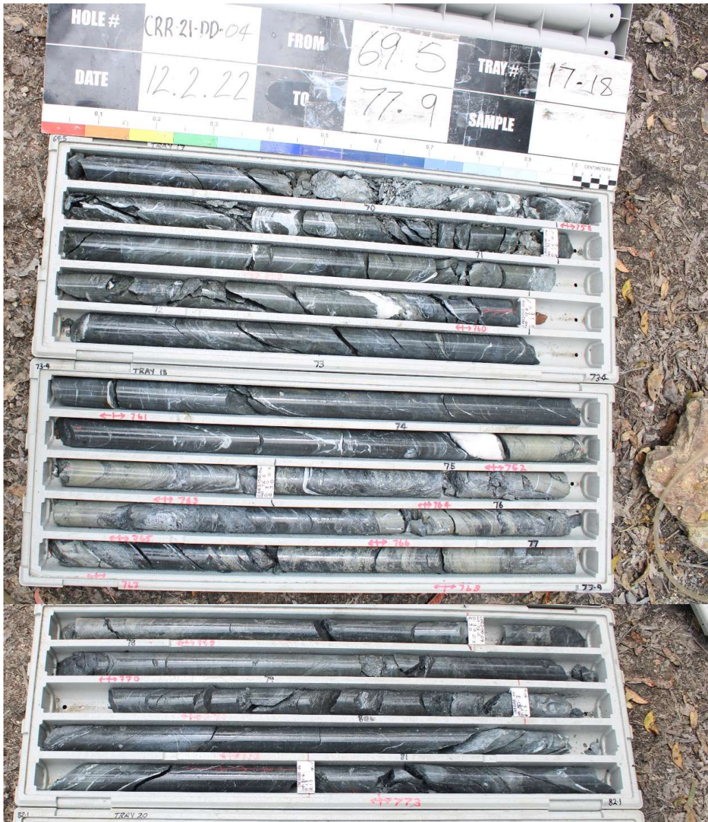
Figure 3: CRR21DD_04. 5.6m interval comprising samples P384762-P384771 assaying at 8.20% Zn, 4.33% Pb, 1.81% Cu, 393.23g/t Ag, 0.51g/t Au from 75.1-80.7m downhole (NQ core, 50mm diameter)
