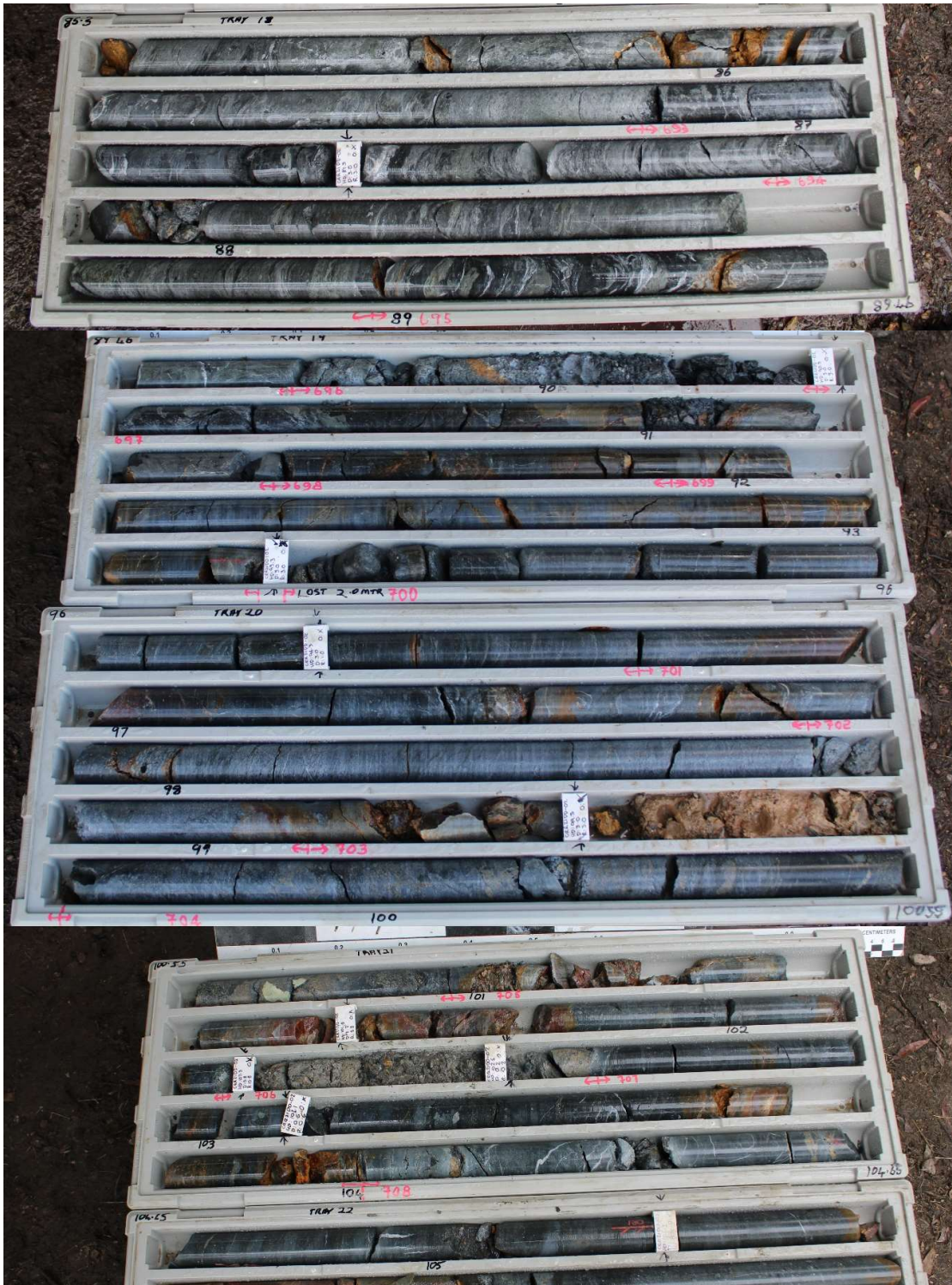
Figure 5: CRR21DD_02, 17.75m interval comprising samples P384649-P384708 assaying at 2.20% Zn, 1.28% Pb, 0.18% Cu, 19.34g/t Ag, 0.09g/t Au from 87.8-105.55m downhole (NQ core, 50mm diameter)
