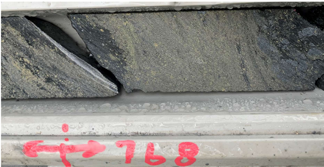
Figure 2: CRR21DD_04, 4.9m interval comprising samples P384745–P384750 assaying at 3.91% Zn, 1.24% Pb, 0.15% Cu, 8.55g/t Ag, 0.04g/t Au, from 58.60-63.5m downhole (NQ core, 50mm diameter)
