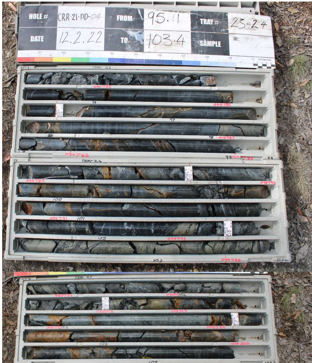
Figure 4: CRR21DD_04, 6.91m interval comprising samples P384787-P384797 ( assaying at 9.41% Zn, 2.45% Pb, 1.56% Cu, 34.6g/t Ag, 0.23g/t Au from 98.04-104.95m downhole (NQ core, 50mm diameter)
