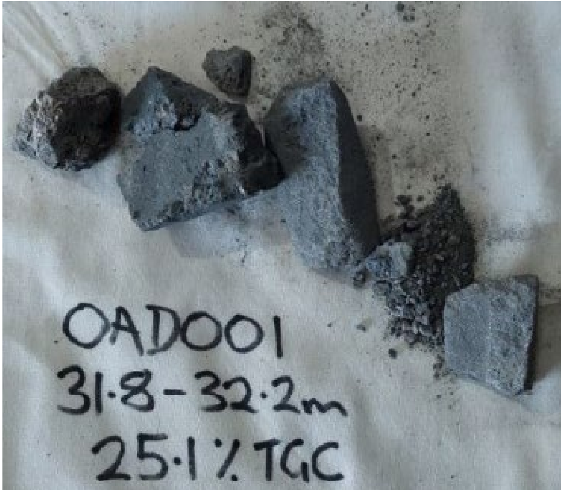
Figure 2: High-grade diamond drill core fragments from OAD001 - resampled for revised testwork 9
