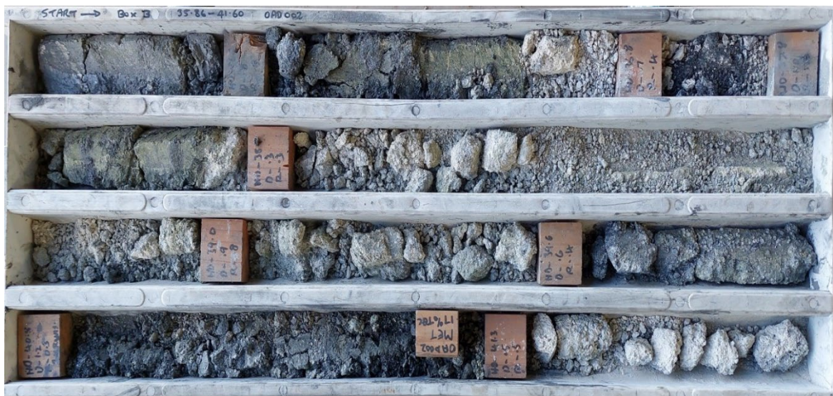
Figure 3: Remaining core from OAD002, (containing 1.7m @ 16.65% TGC from 39.60m), prior to resampling for the revised testwork to feed into the updated scoping study 10
