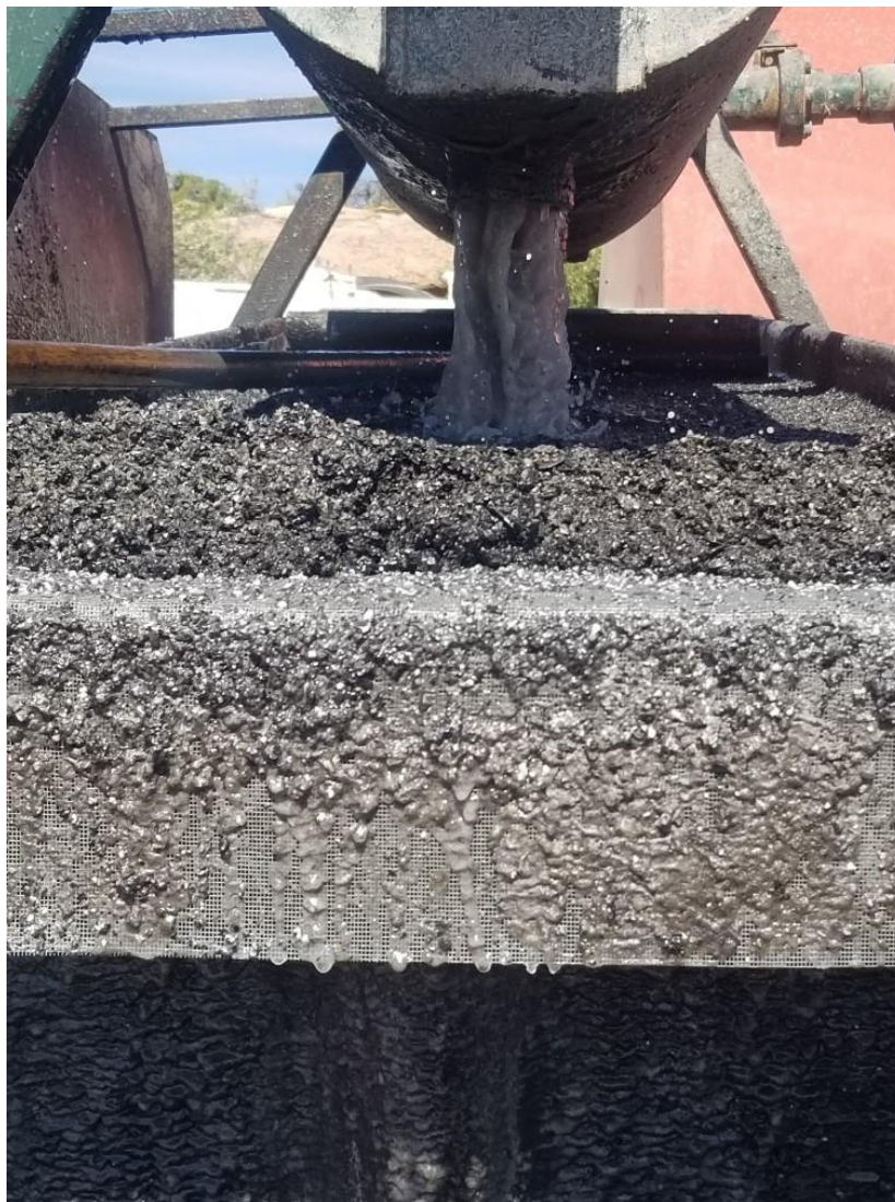
Figure 2: The Mississippian unit drill cuttings which will be sent for petrological examination.
