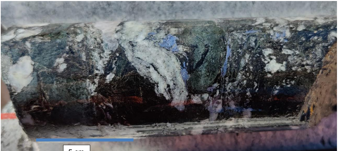
Figure 2. Large “slugs” of grey-blue molybdenite in a zone of fractured quartz veins with associated biotite (dark brown) and chlorite (green).
