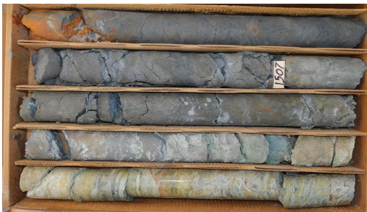
Figure 2: Photo of weathered massive skarn in WD22-19 with abundant iron and zinc oxides between 1501.5 – 1510.5ft (457.6 – 460.3m) downhole. Spot portable XRF readings indicate up to 33.9% Zn (reading at 460.1m).
