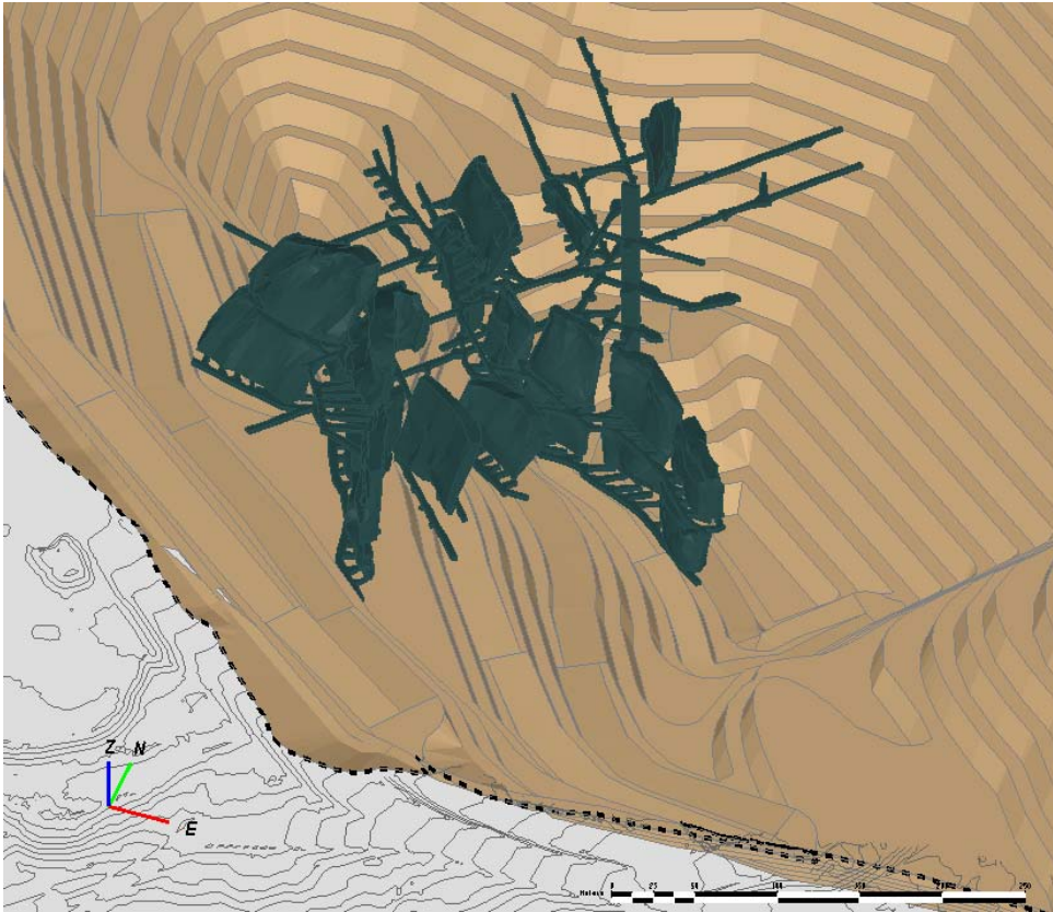
Figure 9: Old Underground Workings
