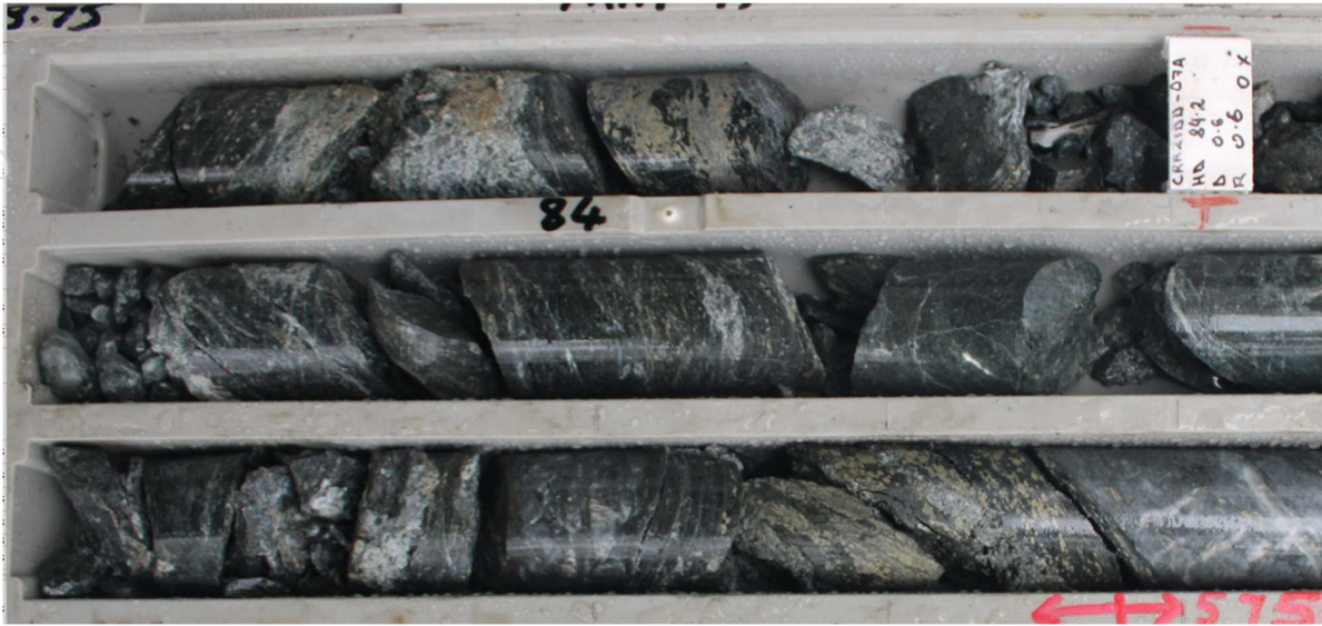
Figure 5: CRR21DD_07A, Portion (all three rows) of sample 42574 comprising carbonaceous black pelite with yellowish-brown sphalerite (zinc sulphide) from a 2.25m downhole interval (83.55-85.80m) assaying 7.52% Zn, 2.92% Pb, 0.32% Cu, 10.7g/t Ag and 0.03g/t Au (NQ core, 50mm diameter)
