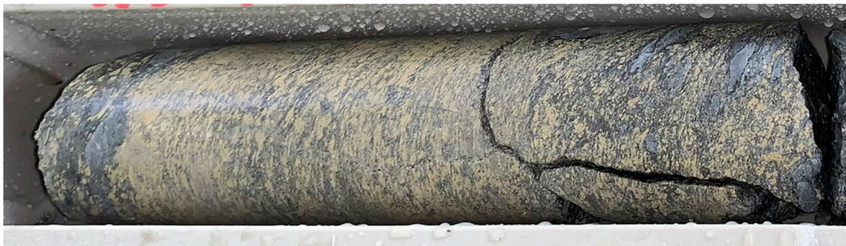
Figure 1: CRR21DD_02A, Portion of sample 384935 exhibiting abundant yellowy-brown sphalerite (zinc sulphide) from sampled downhole interval 73.38-74.38m that assayed 16.7% Zn (NQ core, 50mm diameter)
