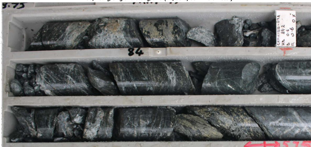
Figure 5: CRR21DD_07A, Portion (all three rows) of sample 42574 comprising carbonaceous black pelite with yellowy-brown sphalerite (zinc sulphide) from a 2.25m downhole interval (83.55-85.80m) assaying 7.52% Zn, 2.92% Pb, 0.32% Cu, 10.7g/t Ag and 0.03g/t Au (NQ core, 50mm diameter)
