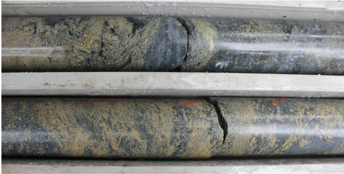
Figure 7: CRR21DD_07A, Portion (both rows) of sample 42583 exhibiting close-up of mineralised breccia with abundant yellowy-brown sphalerite (zinc sulphide) from a 1.9m downhole interval (98.00-99.90m ) assaying 18.35% Zn, 9.08% Pb, 0.94% Cu, 44.5g/t Ag and 0.14g/t Au (NQ core, 50mm diameter)
