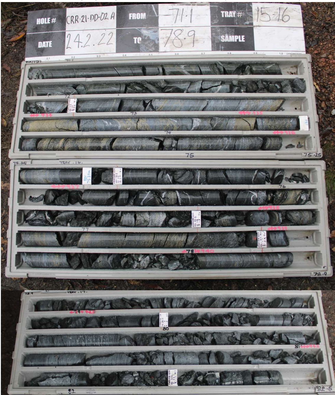
Figure 2: CRR21DD_02A, 6.37m interval comprising samples P384934–P384940 assaying at 7.31% Zn, 0.89% Pb, 0.22% Cu, 10.33g/t Ag, 0.08g/t Au, from 72.65-79.02m downhole (NQ core, 50mm diameter)
