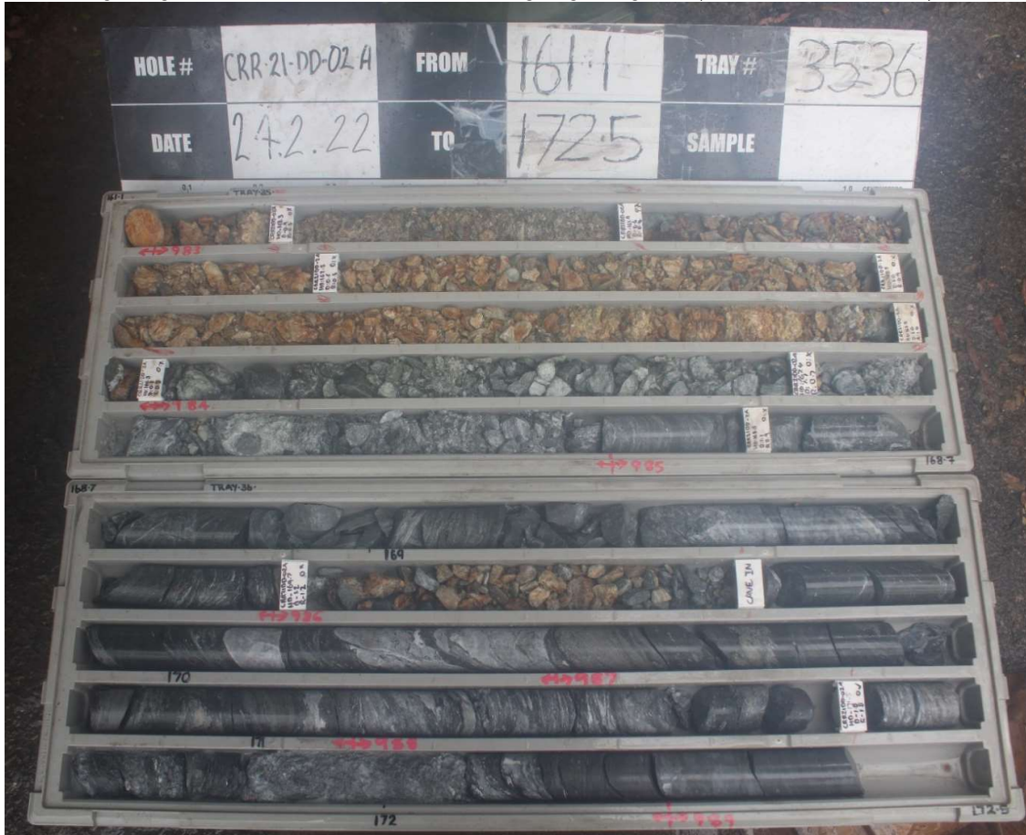
Figure 3: CRR21DD_02A. 5.3m interval comprising samples P384984-P384987 from 166.3-171.6m depth downhole, grading 4.10% Zn, 1.78% Pb, 0.49% Cu, 25.17g/t Ag, 0.09g/t Au. (NQ core, 50mm diameter)
