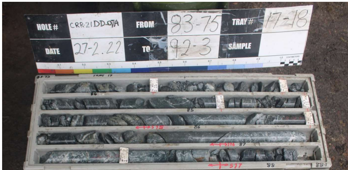
Figure 4: CRR21DD_07A, 3.35m interval comprising samples 42574 -42575 from 83.55-86.9m downhole assaying 6.06% Zn, 2.06% Pb, 0.23% Cu, 7.86g/t Ag, 0.02g/t Au (NQ core, 50mm diameter)
