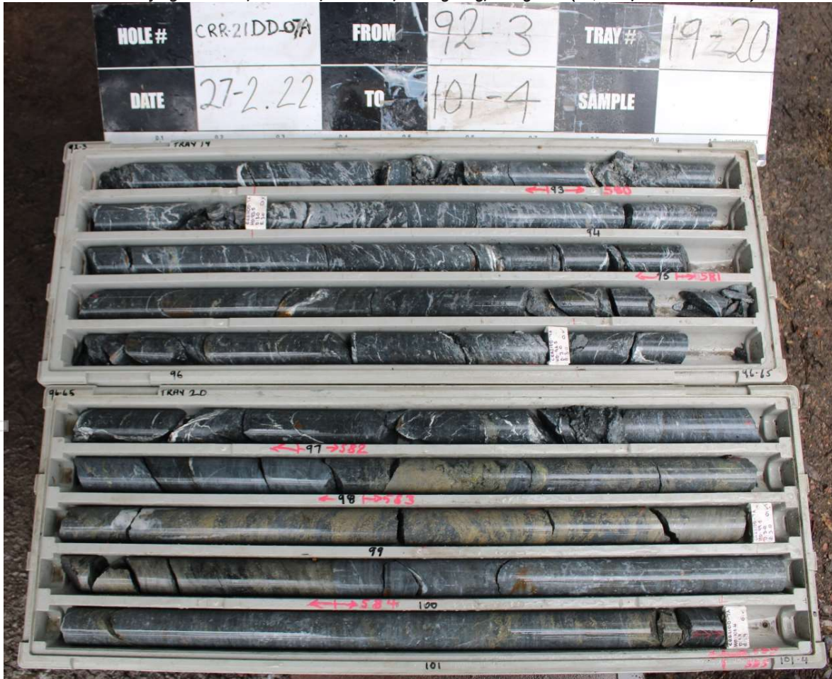
Figure 6: CRR21DD_07A, 4.5m interval (second tray) comprising samples 42583-42585 from 98-102.5m downhole assaying 9.22% Zn, 4.34% Pb, 0.98% Cu, 23.81g/t Ag, 0.08g/t Au (NQ core, 50mm diameter)
