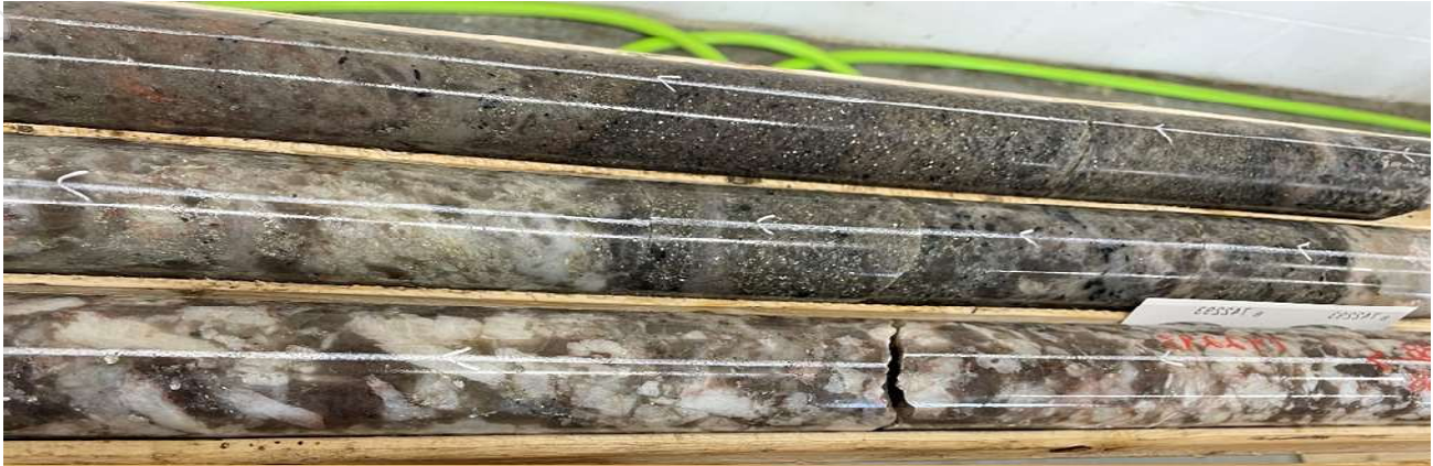
Figure 2: Close up images of large silvery-white coloured spodumene crystals intercepted in Hole MF22-73 (Hole 14)
