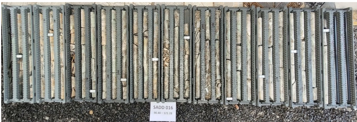
Figure 2: SADD016, 91.60 – 119.38m, 27.28m pegmatite with large fresh light green spodumene crystals throughout
