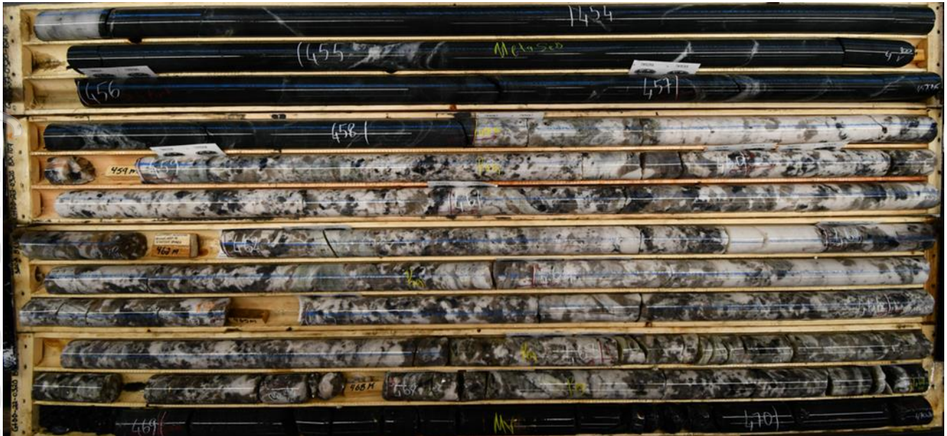
Figure 4: Diamond drill core from hole GTDD-22-0320; thick, high-grade LCT spodumene bearing pegmatite intercept of 10.7m from 458.2m
