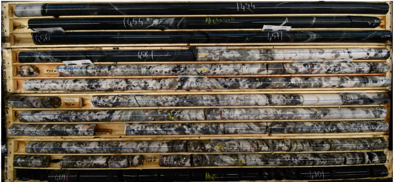
Figure 4: Diamond drill core from hole GTDD-22-0320; thick, high-grade LCT spodumene bearing pegmatite intercept of 10.7m from 458.2m
