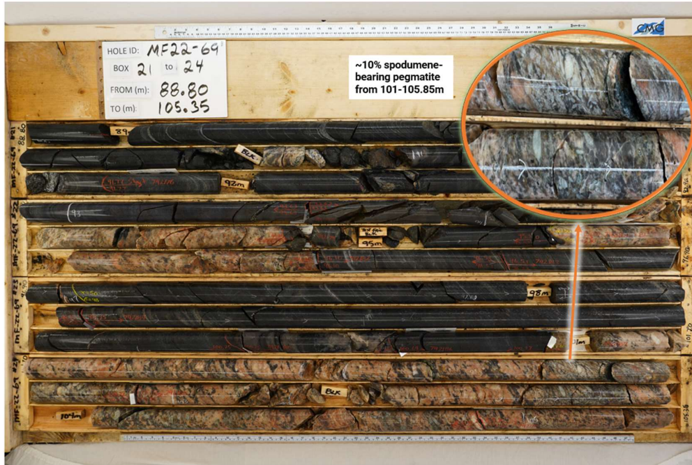
Figure 6: A significant intercept of white to grey pegmatite hosts approximately 10% of medium to large, white grey, spodumene crystals intersected from 101-105.85 metres downhole in Hole MF22-69 (Hole 10). Close ups illustrate significant spodumene mineralisation
