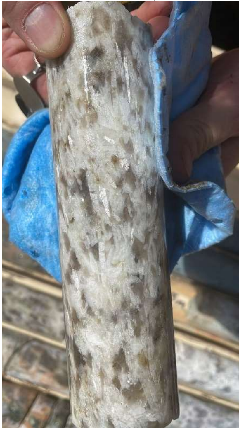
Figure 2: Core comprising almost entirely of spodumene laths. Visual estimates were as high as 60% in metre-scale intervals in Hole MF22-72 (Hole 13)
