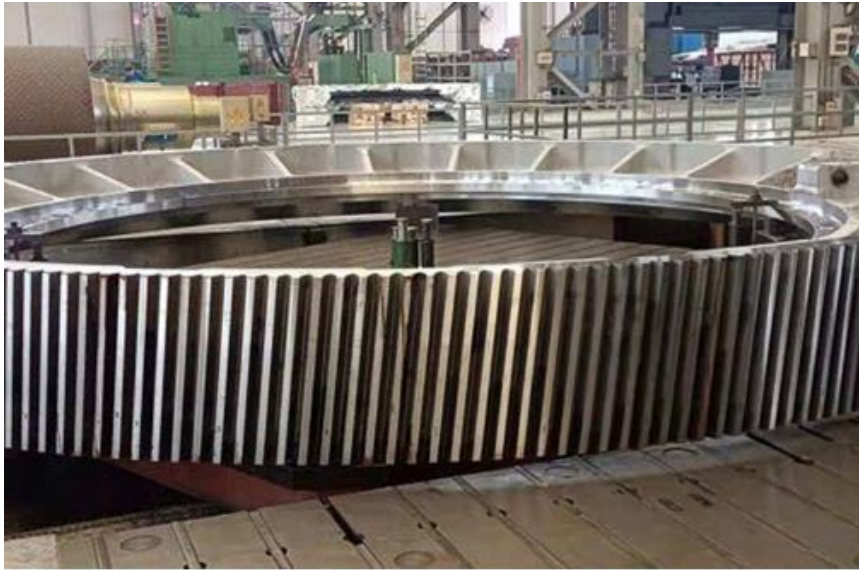
Figures 12 – New mill girth gear nearing completion.
