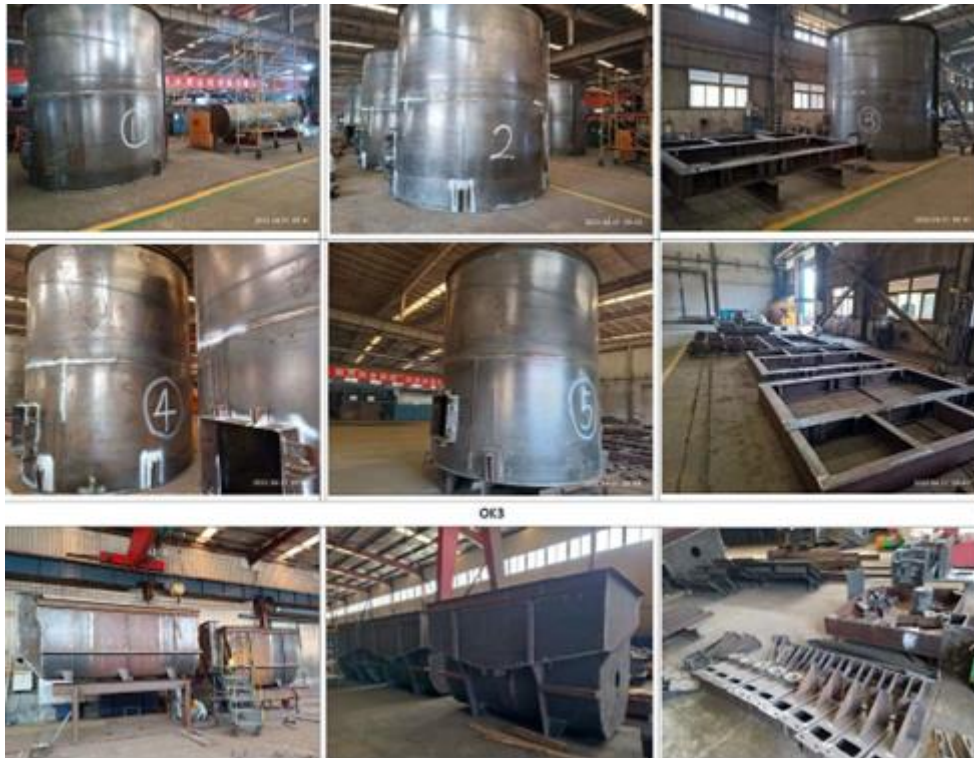
Figure 10 – Flotation cell fabrication.
