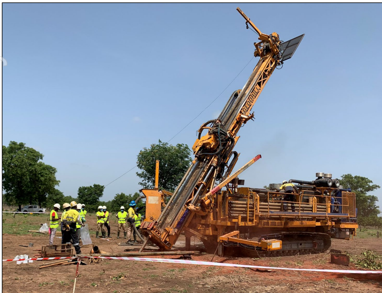
Figure 4: RC drill at commencement of maiden drilling program at the Korhogo Project.
