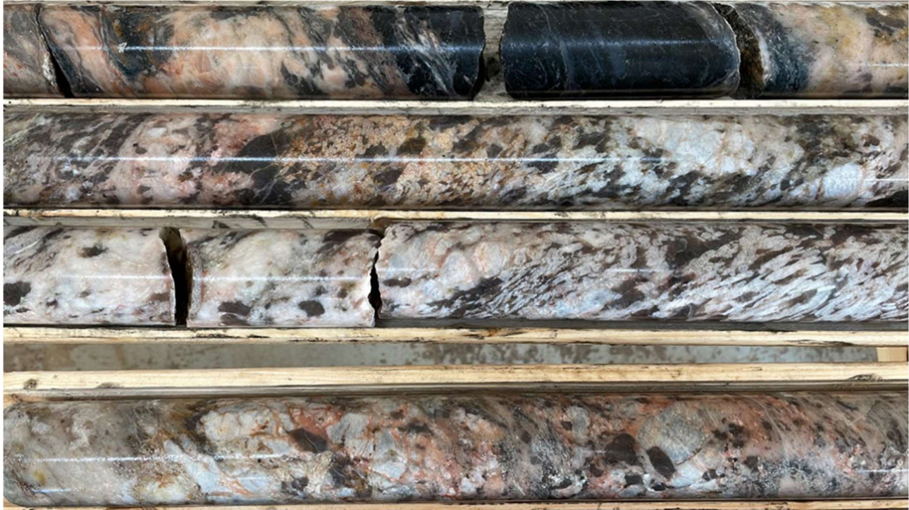
Figure 1: Close up images of large cream coloured spodumene crystals intercepted in Hole MF22-66 (Hole 7)
