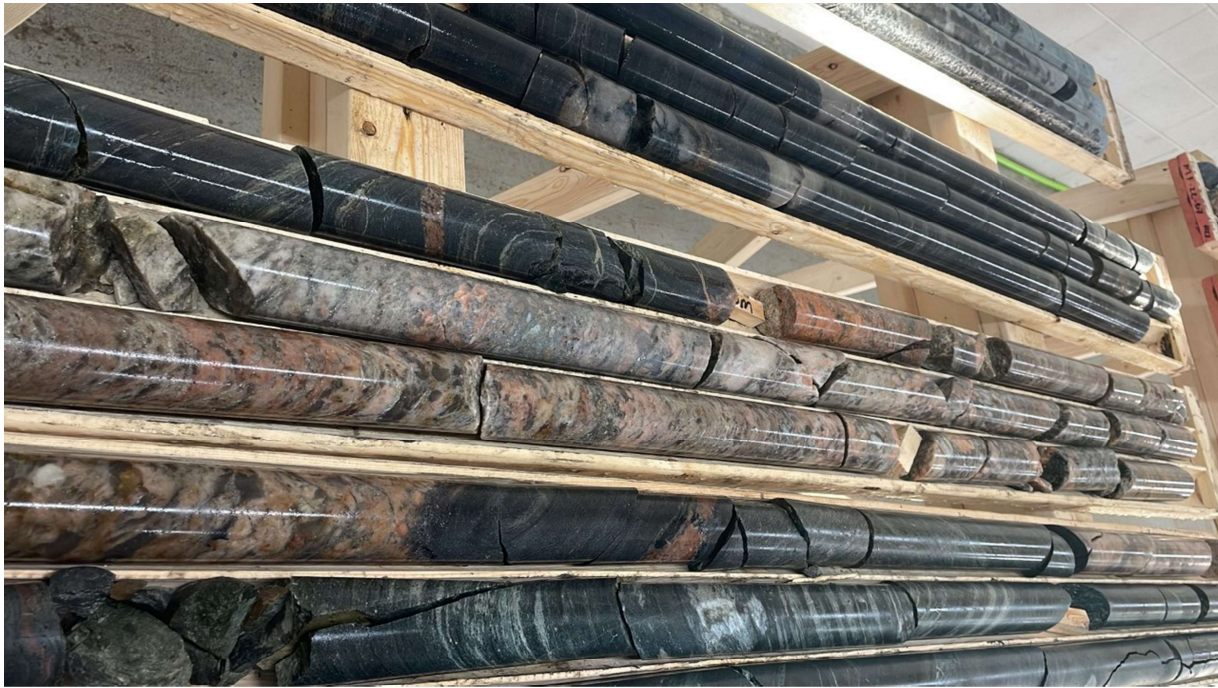
Figure 5: Close up of white to grey-pink pegmatite hosts approximately 5% of medium, white grey, spodumene crystals intersected from 83-86.77m downhole in Hole MF22-67 (Hole 8)
