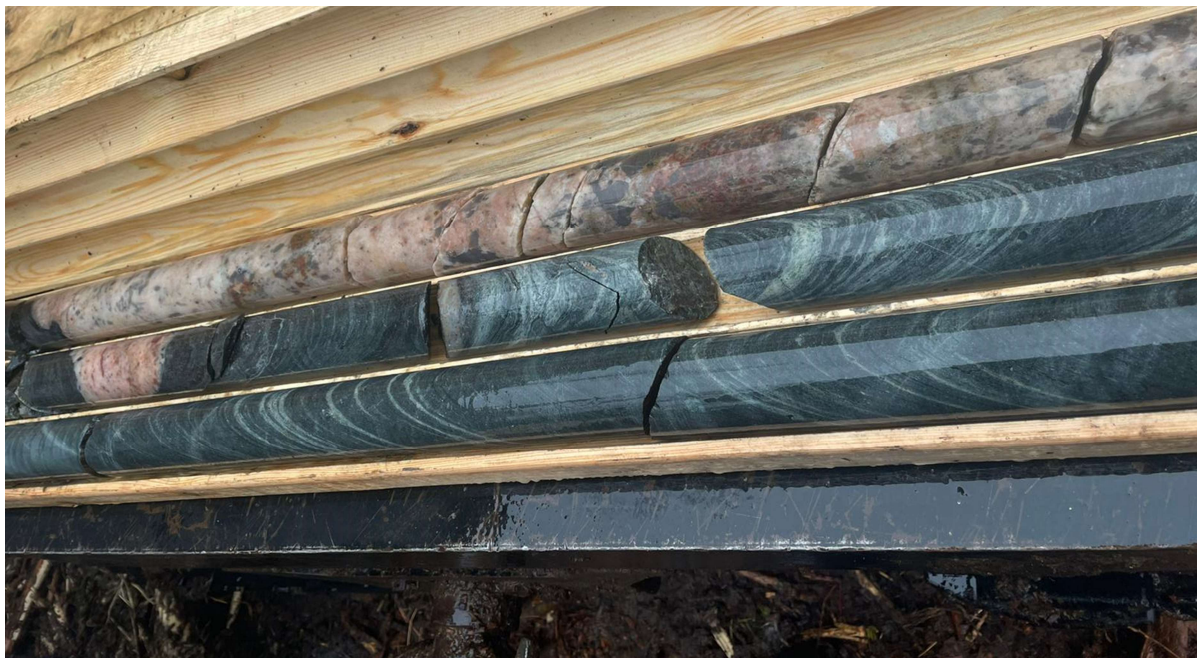
Figure 6: Close up of white to grey pegmatite that hosts approximately 5% of medium, white grey, spodumene crystals intersected from 83.62 to 84.5m downhole in Hole MF22-68 (Hole 9)
