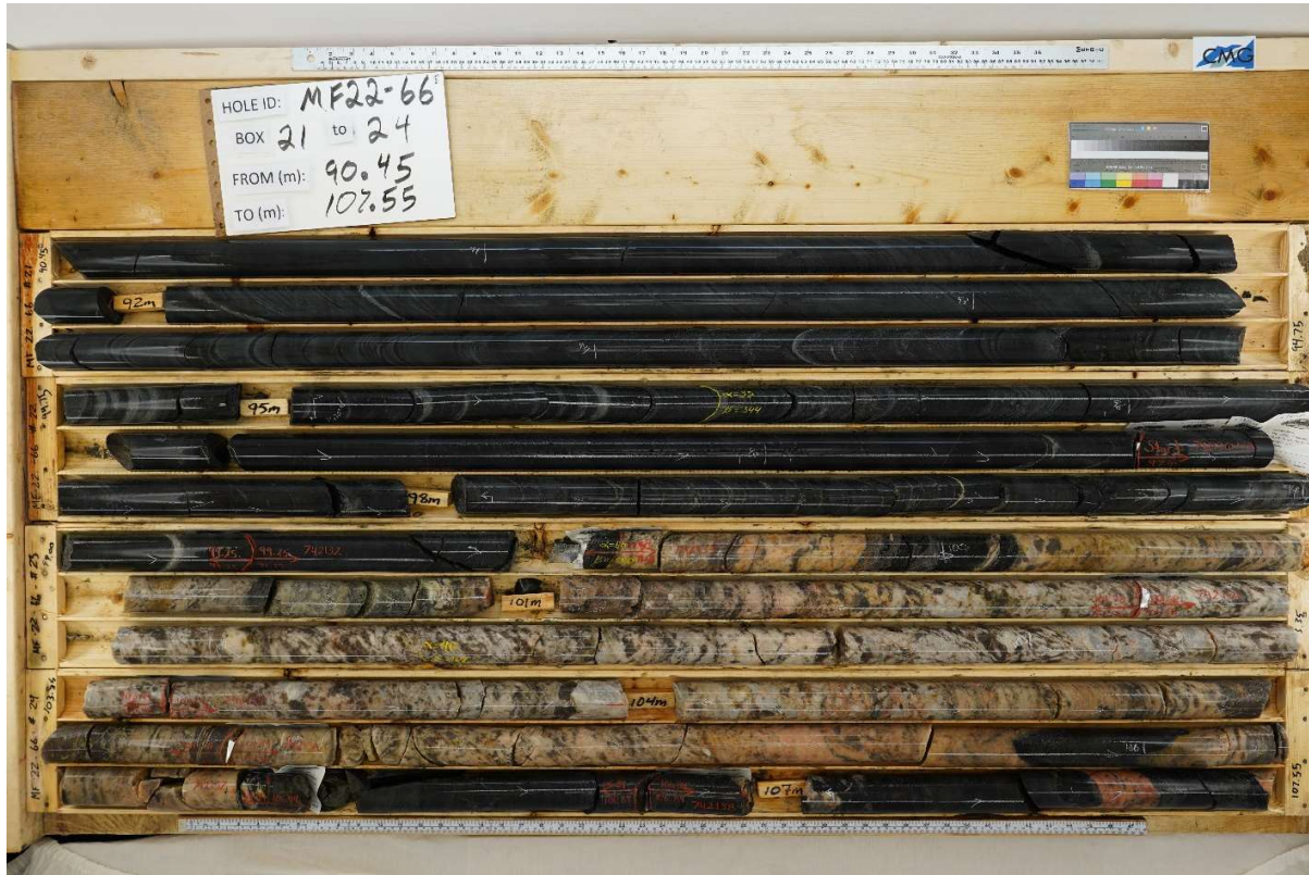
Figure 4: White to grey pegmatite hosts approximately 20% of medium to large, white grey, spodumene crystals intersected from 99.6-106.5 metres downhole in Hole MF22-66 (Hole 7)
