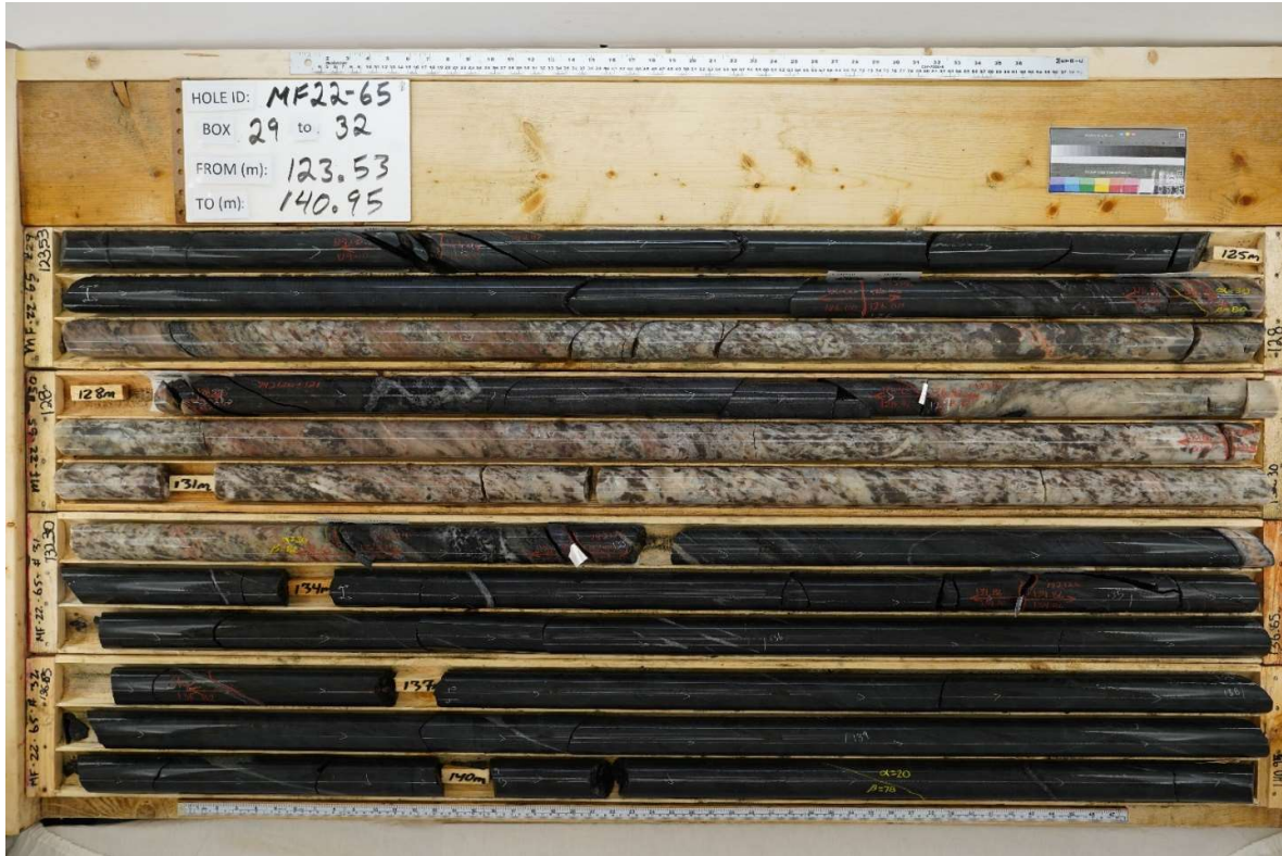
Figure 2: A significant intercept of white to grey pegmatite hosts approximately 30% of medium to large, white grey, spodumene crystals intersected from 126.4-128 and 129-132.6 metres downhole in Hole MF22-65 (Hole 6).
