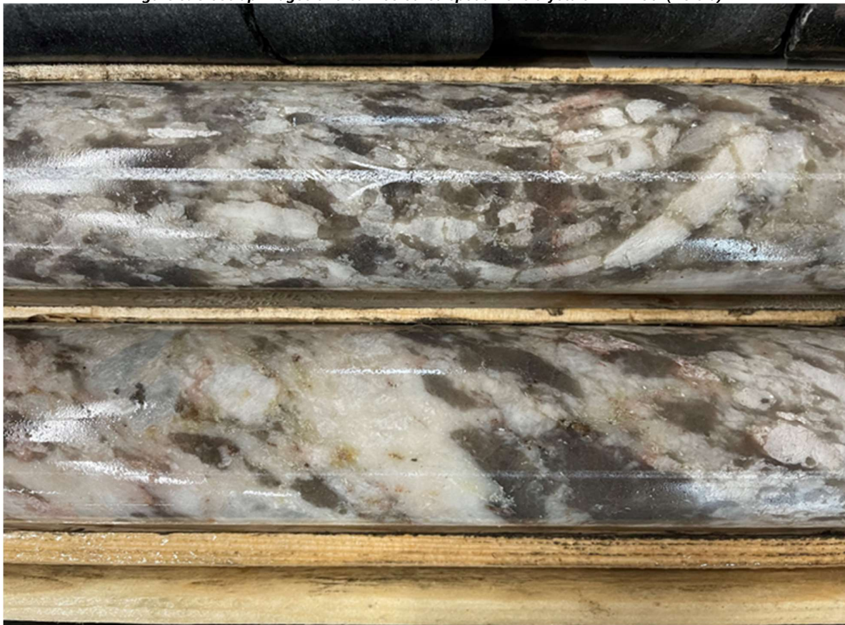
Figure 3: Close up images of cream coloured spodumene crystals MF22-65 (Hole 6)
