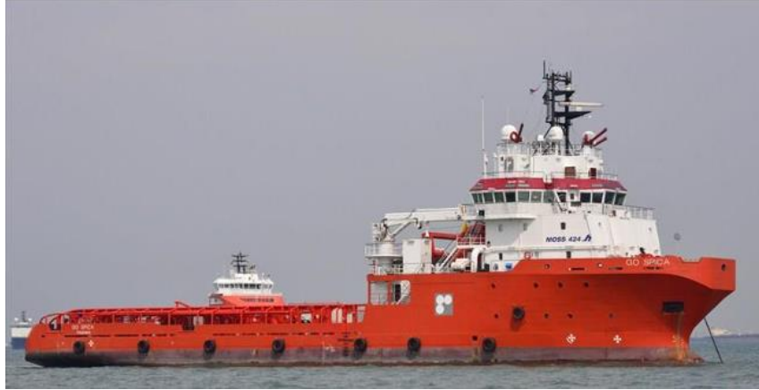
GO Offshore GO Spica Anchor Handling Tow Vessel (AHTV)
