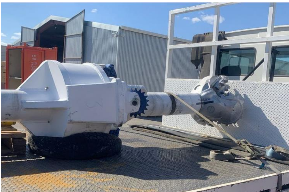
Hole Opener 26" Bit x 42" Hole Opener
