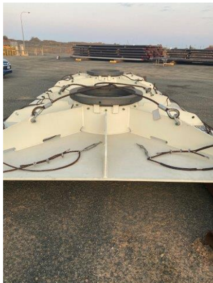
Mud Mats for Conductor Support
