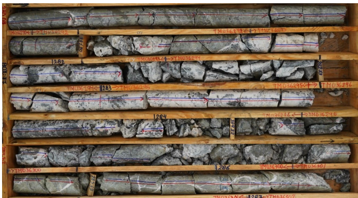
Figure 3: A photograph of mineralised interval in drill hole CVD057, averaging 3.45g/t gold over 8.39m from 278.61m. The mineralised interval is centered around a 6.80m quartz-carbonate breccia averaging 4.04g/t gold
