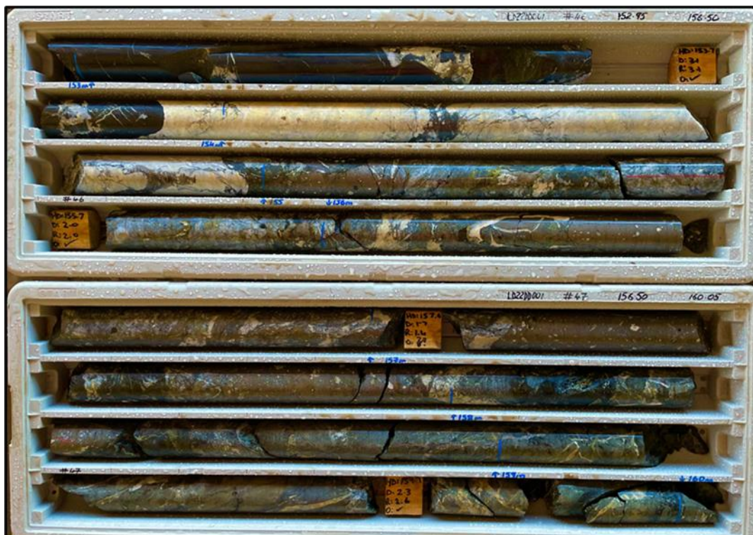
Figure 4 Mineralised drill core from LD22DD001 from 153 – 160m showing massive sulphides with chalcopyrite and pyrrhotite mineralised matrix-supported hydrothermal breccia and quartz – carbonate breccia and veining in a shale unit.
