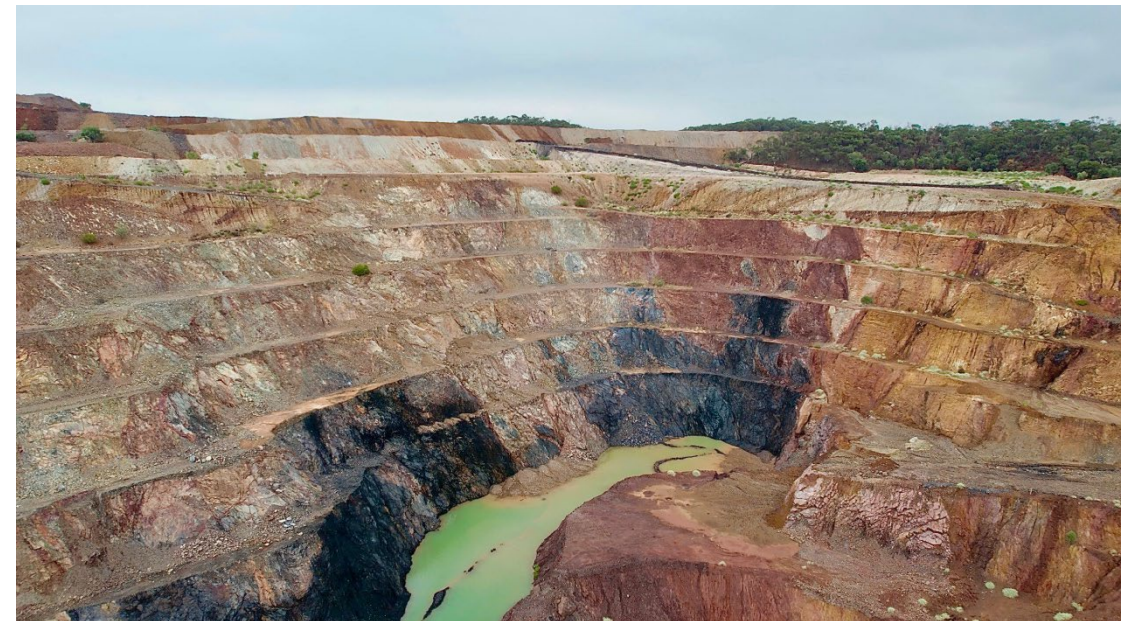
Flying horse pit showing progression from oxide at top of pit to transition then fresh or sulphide material at the bottom of pit
