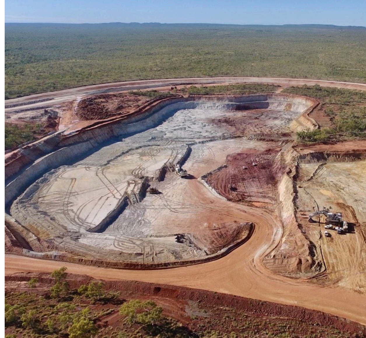
Mining at east pit 27 Apr 22. Ore can be seen on RHS of pit as darker coloured material.
