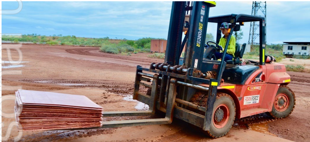
Taking new cathode bundle to be sampled, strapped and wrapped for shipment.
