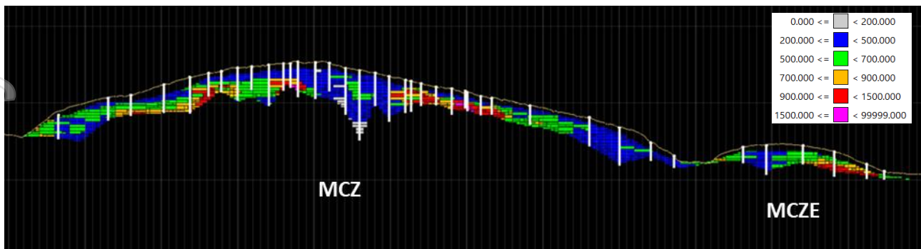
Figure 6: Makuutu Rare Earths Project – Cross section 57,400N (looking north) with TREO block grades (10x vertical exaggeration)
