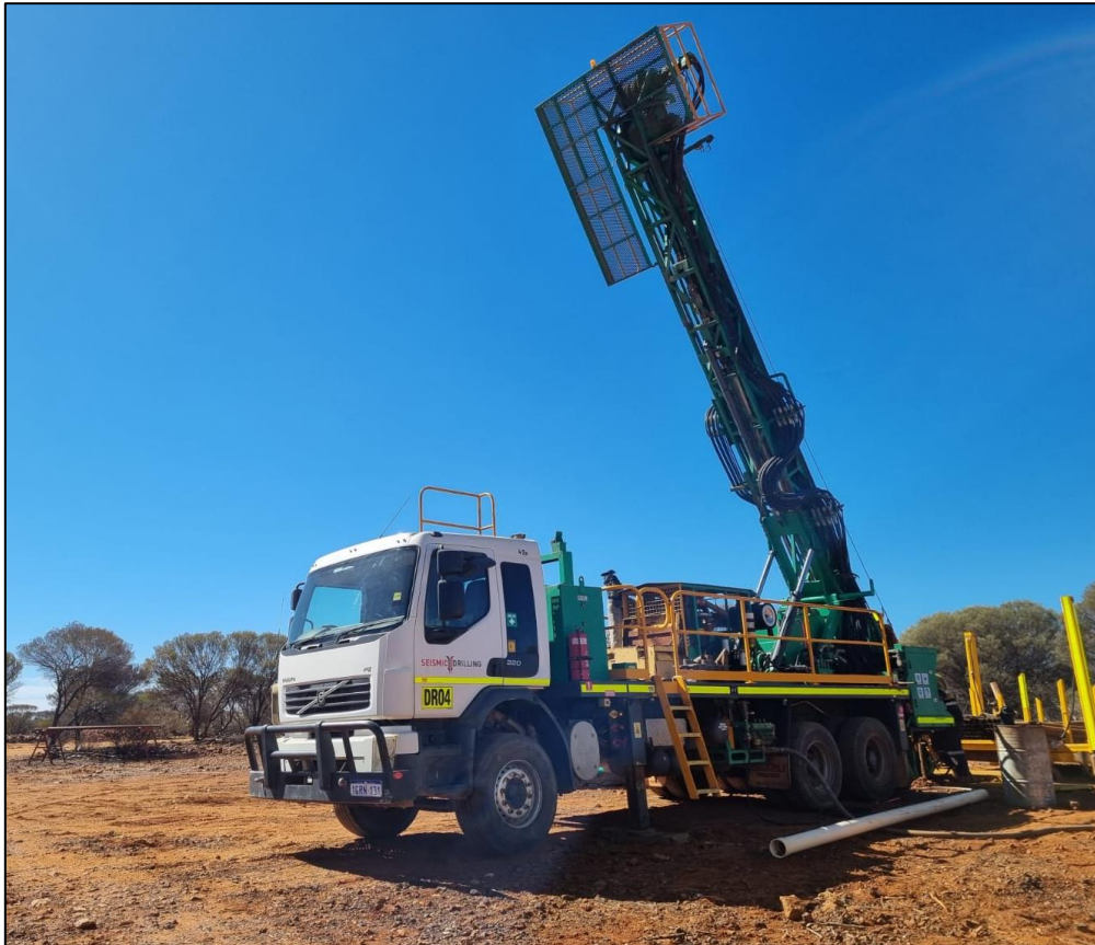
Photograph 1 – Seismic Drilling Australia Pty Ltd DR04 on site at Leinster Nickel Project
