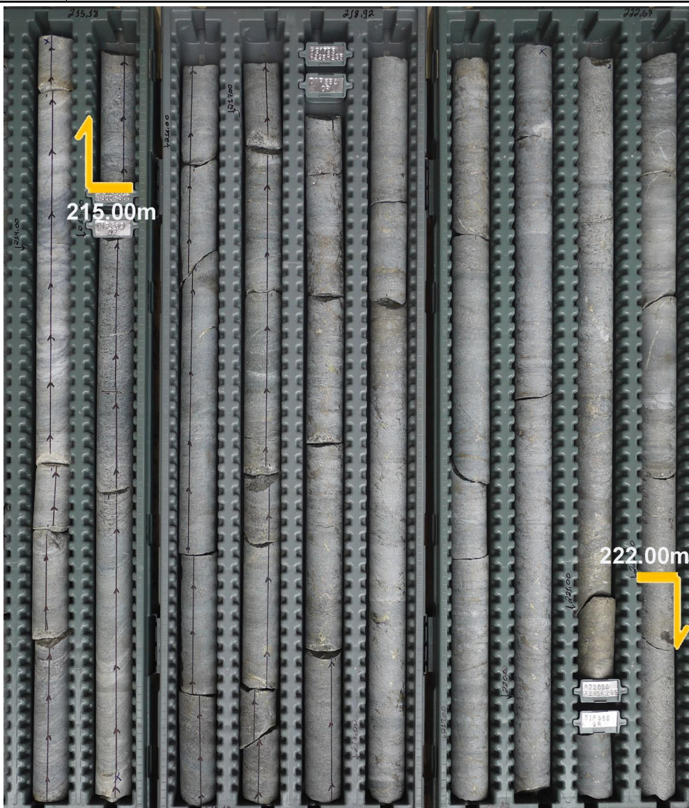
Drill core photo from PD3-016:7.00m @ 1.01% Cu, 0.47% Zn, 0.05% Pb, 6.14g/t Ag, 0.04g/t Au from 215.00m. Mineralised interval is between the orange markers.
