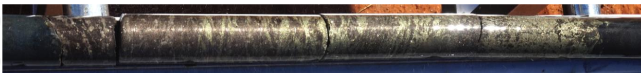
Figure 2. High grade massive sulphide from PSD02. The sulphide has a conductance in excess of 5,000 siemens and similar to that modelled for the new conductor.
