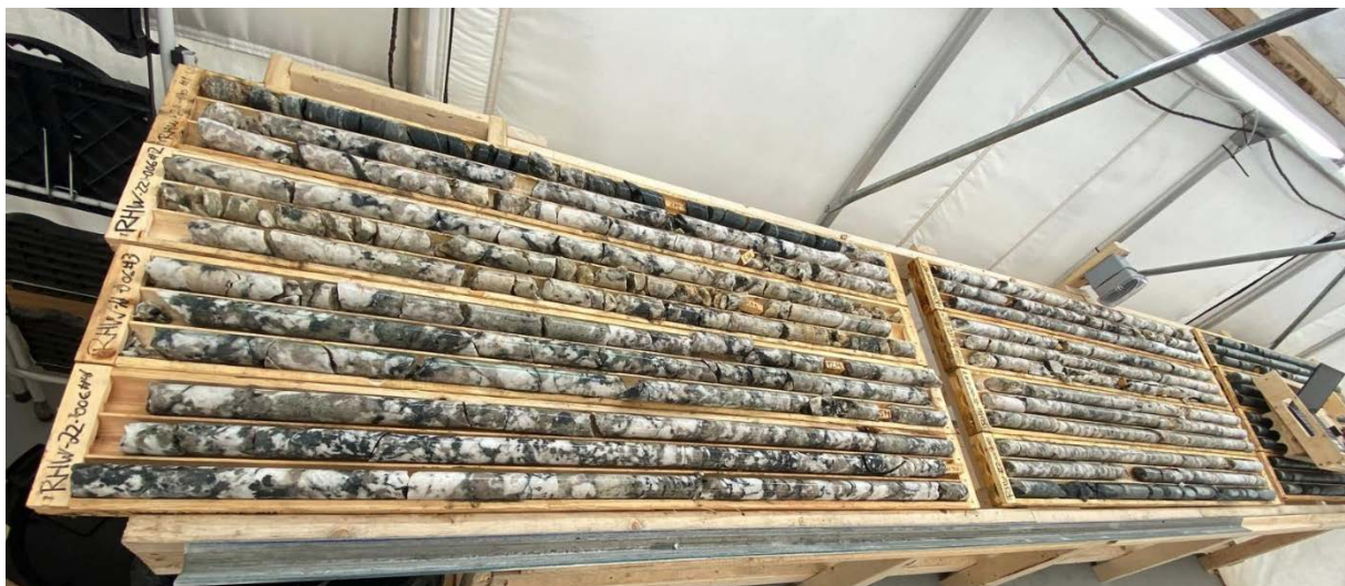
Figure 1: 31.2m of spodumene bearing pegmatite in core, Ruby Hill West drilling starting at 3.5m in RHW22-006
