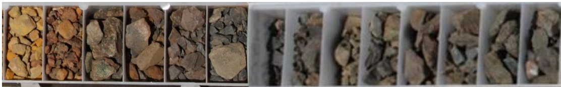
Image 7 / RC drill chips: 21MDWB02 34-48m (14m @ 0.81% Cu & 366ppm Co. malachite & cuprite mineralisation)
