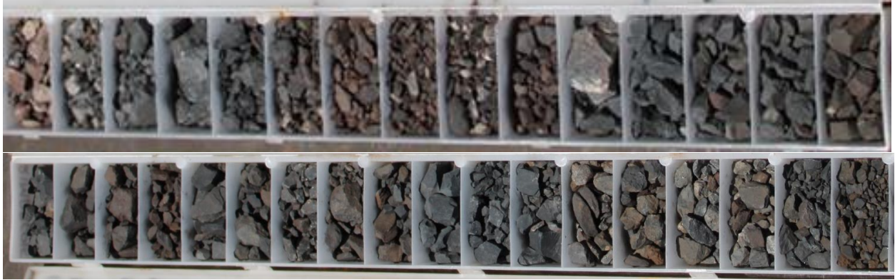
Image 3 / RC drill chips: 21MDRC015 65-76m (11m @ 2.27% Cu & 429ppm Co & 78-98m 20m @ 1.99% Cu & 30ppm Co, chalcocite & covellite mineralisation)
