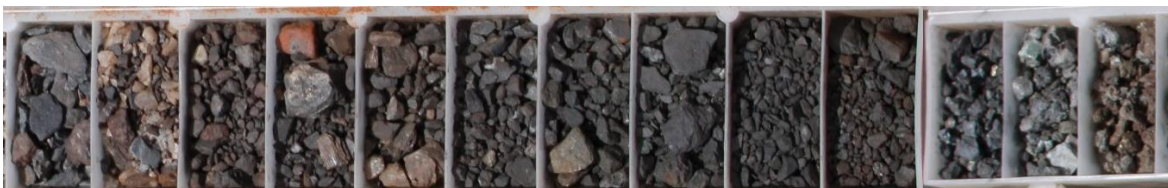
Image 2 / RC drill chips: 21MDRC012, 50-63m (13m @ 0.85% Cu & 429ppm Co, cuprite, chalcocite & covellite mineralisation)
