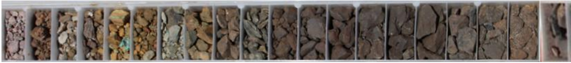
Image 4 / RC drill chips: 21MDRC016 41-61m (20m @ 0.86% Cu & 609ppm Co malachite, cuprite & chalcocite mineralisation)
