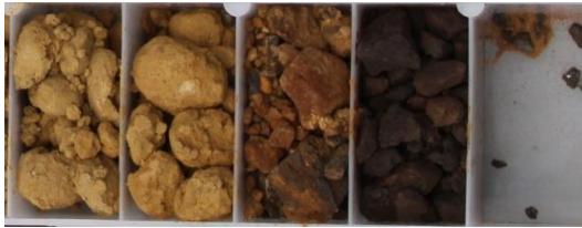
Image 5 / RC drill chips: 21MDRC017 34-39m (5m @ 1.68% Cu & 678ppm Co cuprite mineralisation)
