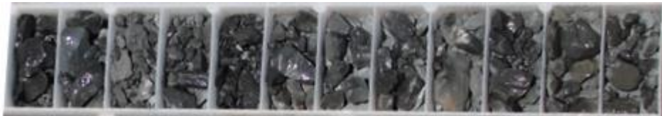
Image 6 / RC drill chips: 21MDRC018 108-117m (9m @ 0.95% Cu & 284ppm Co. pyrite & chalcopyrite mineralisation)
