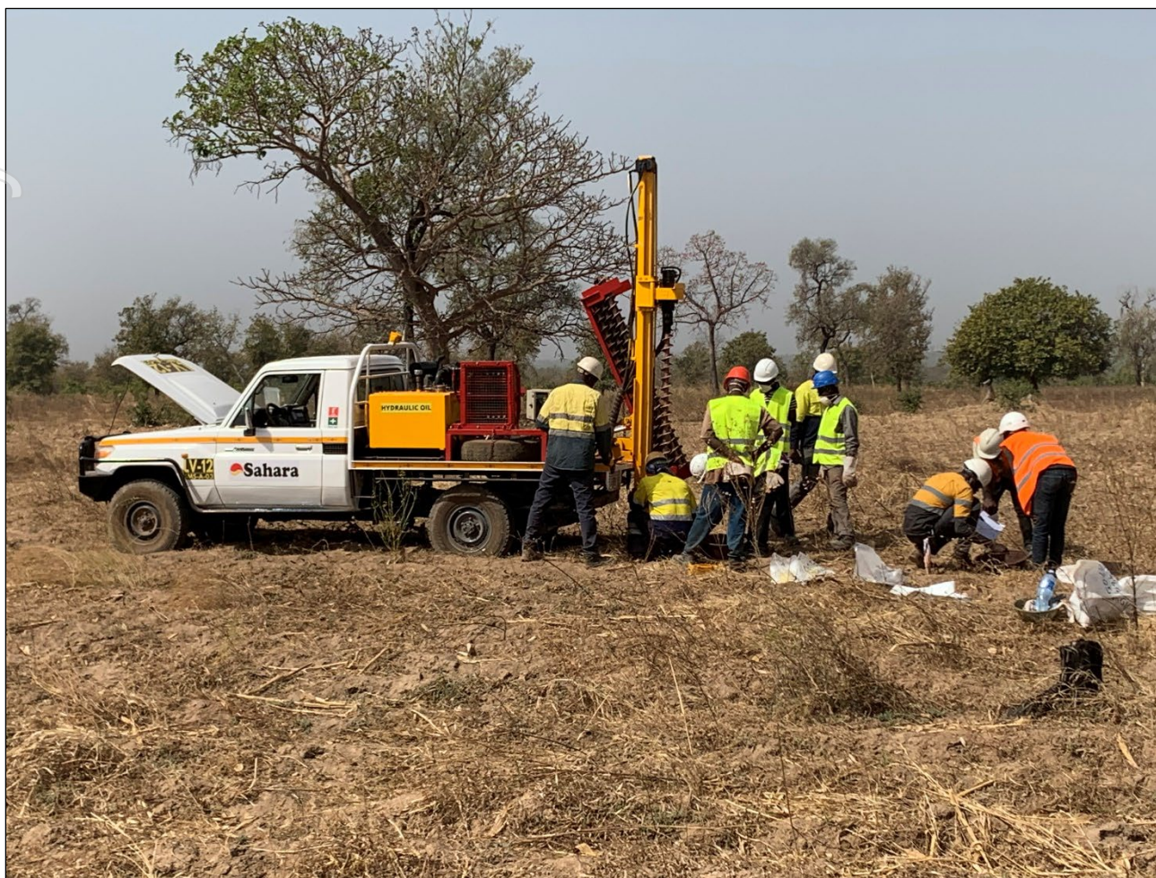
Figure 10: Auger drill on the Korhogo Nord permit
