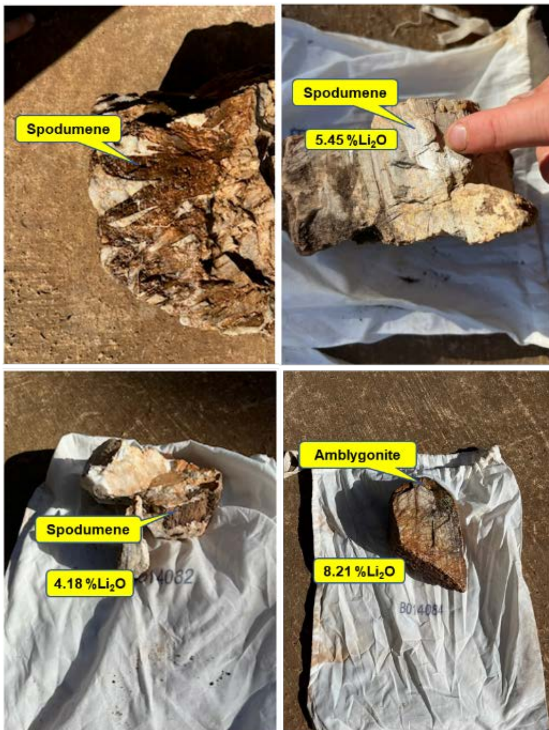
Figure 2: Lithium mineralisation at Big pegmatite
