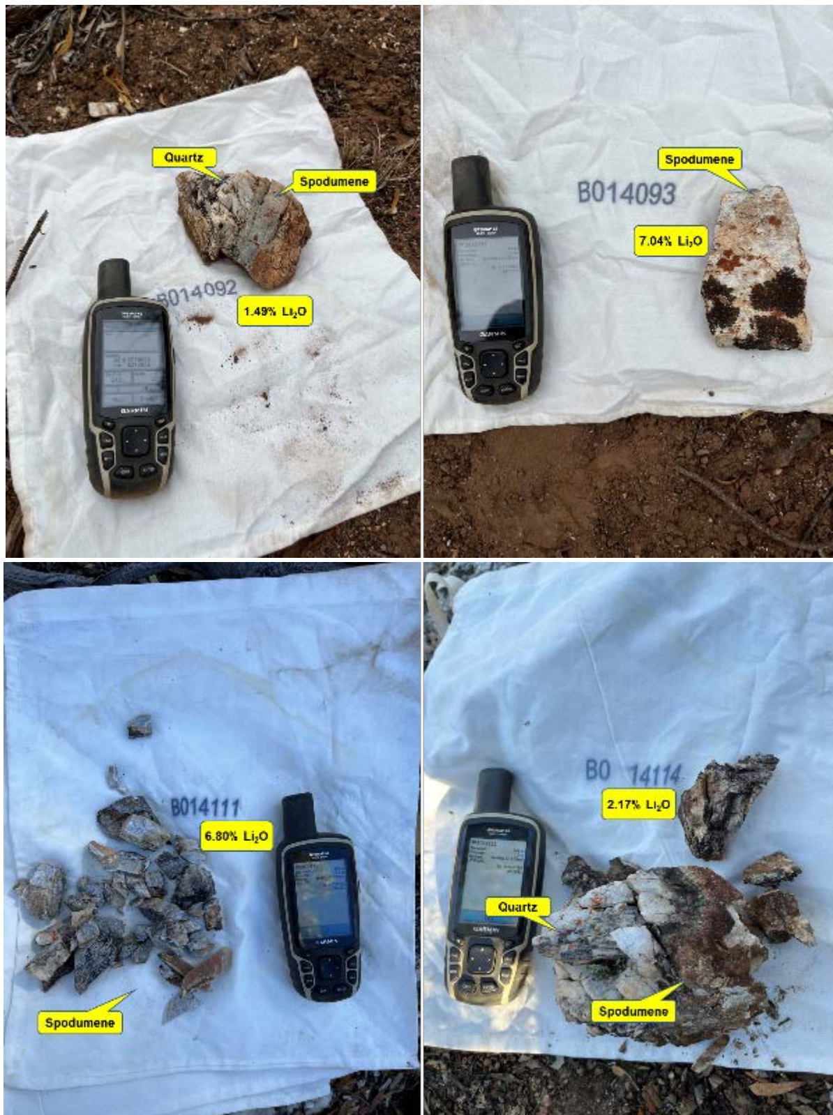
Figure 3: Spodumene lithium mineralisation north and southwest of Big pegmatite
