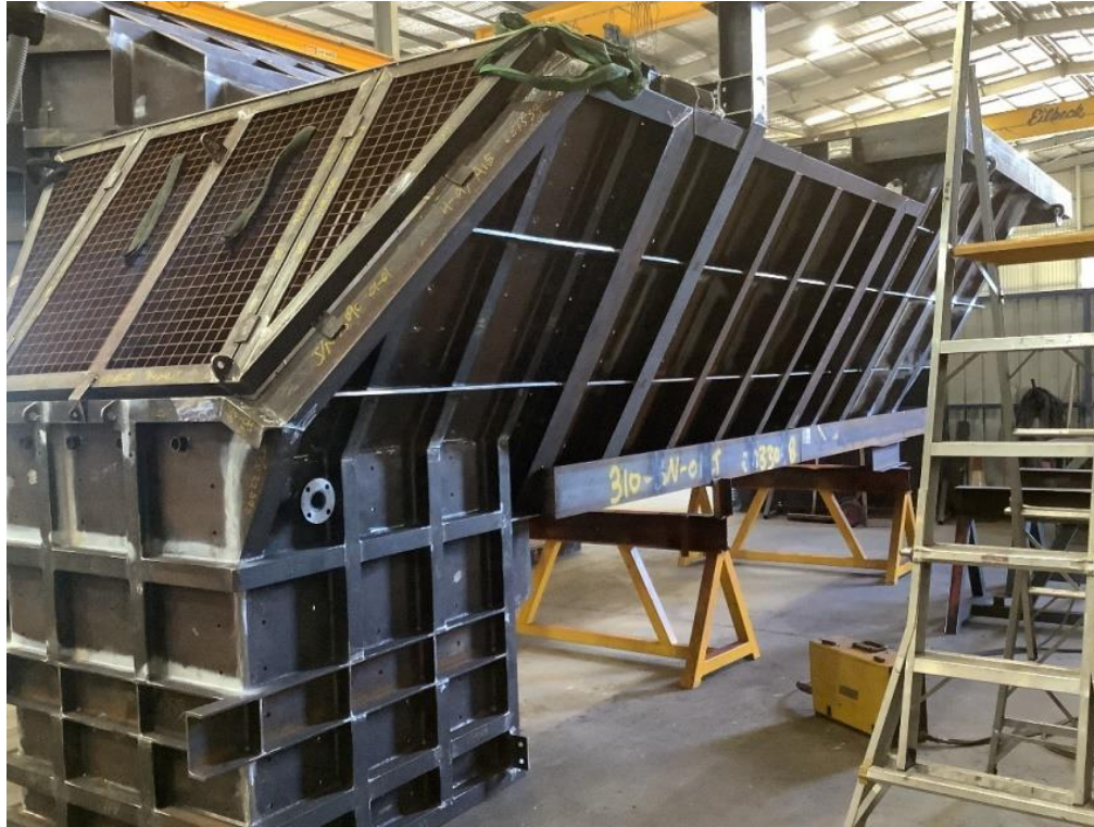
Figure 8. Primary crusher feed chute fabrication (Perth).
