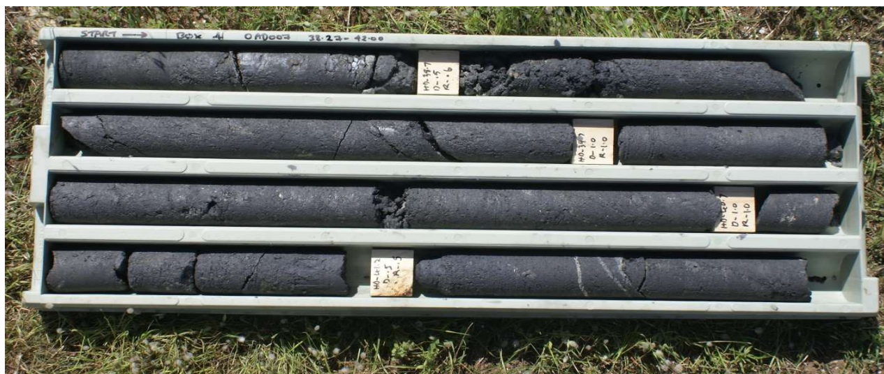
Figure 2: High-grade graphite drill core from the Oakdale Graphite Project – 36.2m to 42.2m @ 19.71% TGC 5
