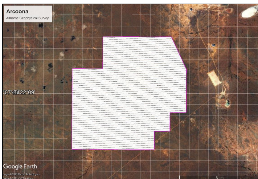
Figure 6: Arcoona approx. 4600-line kilometer fixed-wing airborne magnetics survey area. The survey was designed to cover most of the tenement where potential for greenstones under cover has been identified. Please refer to previous ASX announcement (12 April 2022) for further details.
