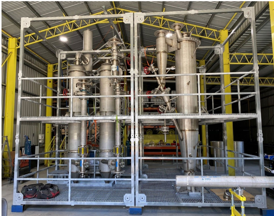
Fluid Bed Reactor pilot plant testwork being undertaken in Glen Innes
