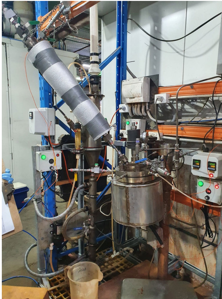
Iron hydrolysis testwork at Simulus
