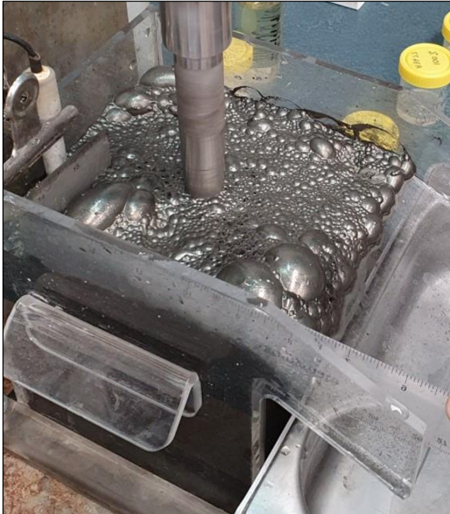
Figure 1 – Nickel concentrate (>13% Ni) produced during testwork on the high-grade massive nickel sulphides from Sample 3 (source: internal report from Strategic Metallurgy)
