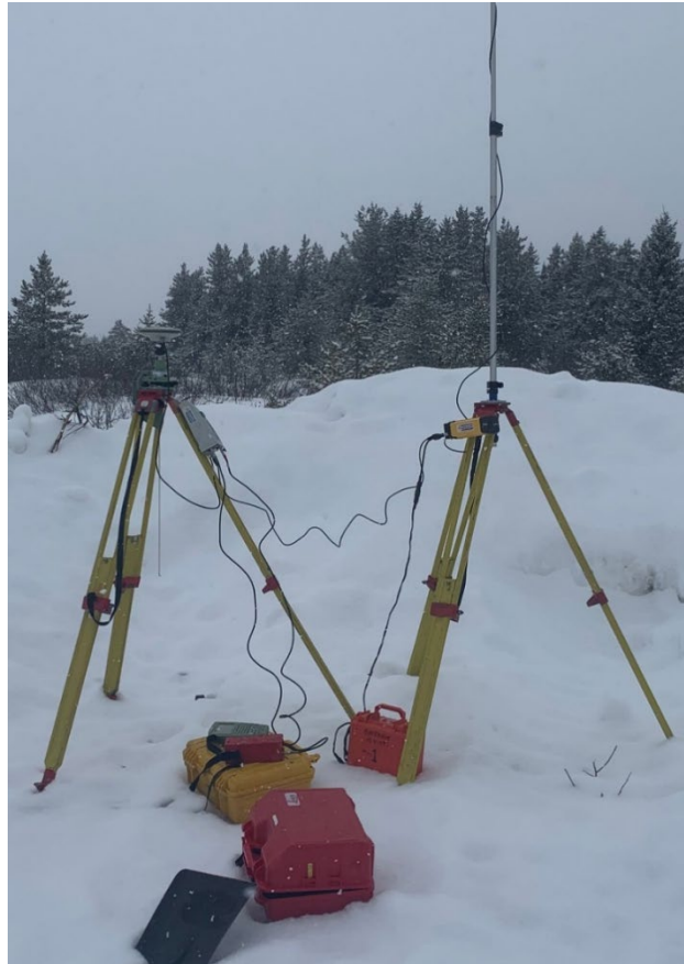
Figure 8 – Gravity base station set up
