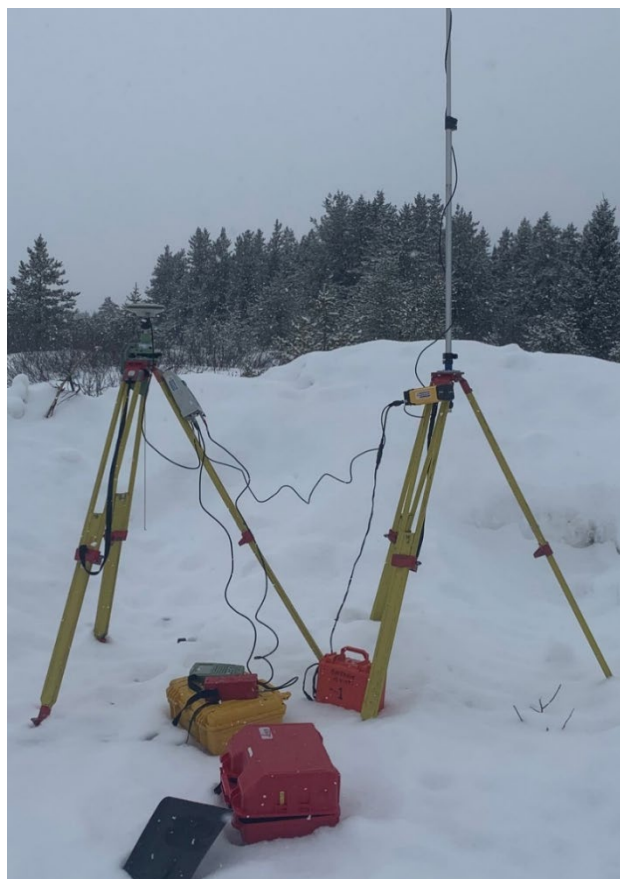
Figure 8 – Gravity base station set up
