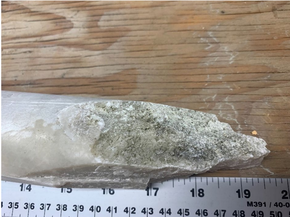
Figure 7 – Spodumene crystals are visible in pegmatites detected in initial drill core
