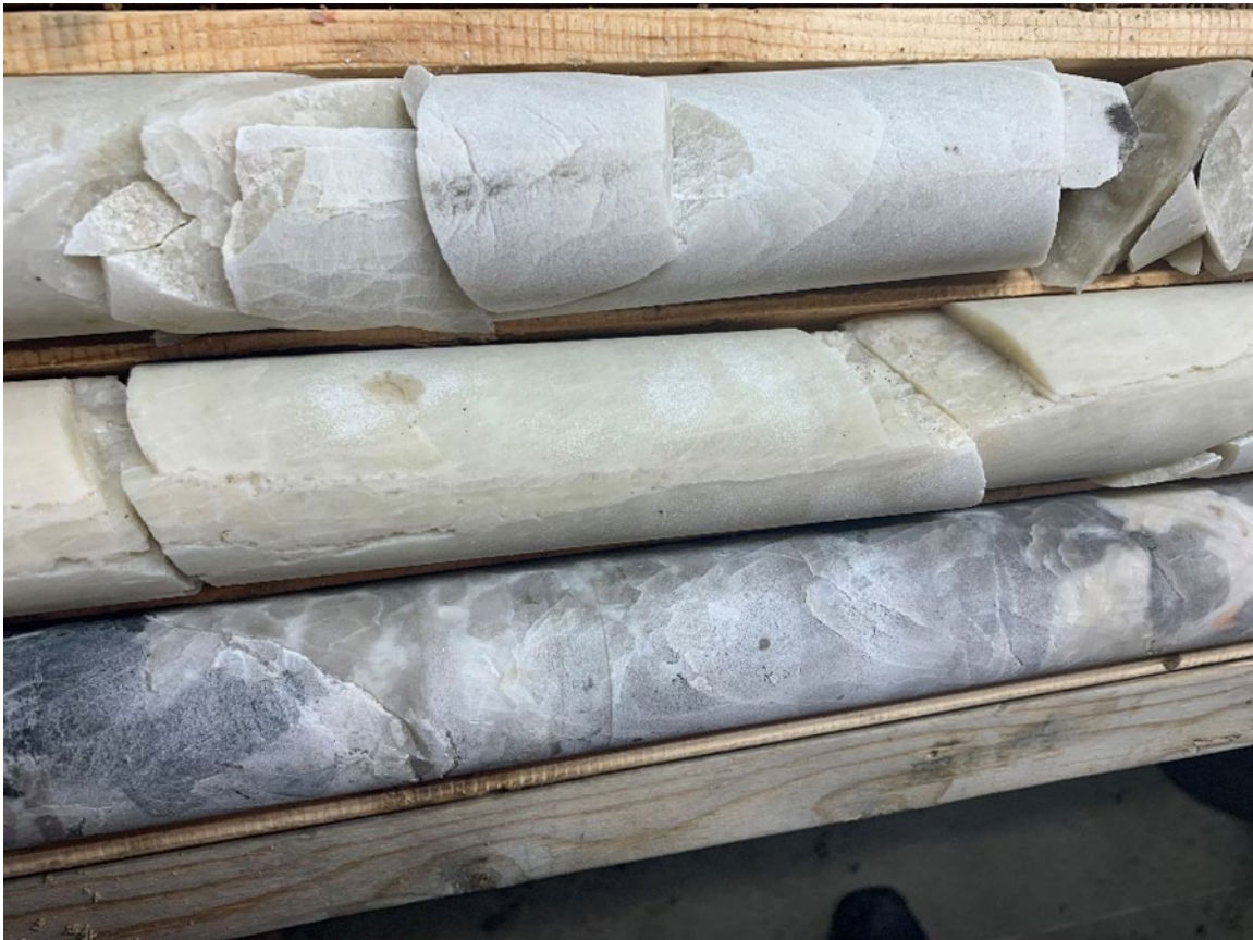
Figure 6 - Visible spodumene crystals have been detected in the initial drill core
