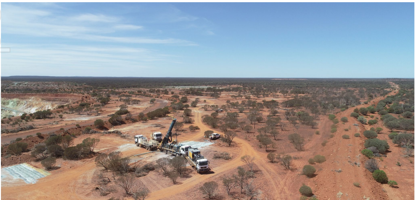
Figure 2: RC drilling at Lord Nelson (looking south-east), southern end of the pit can be seen on the left.
