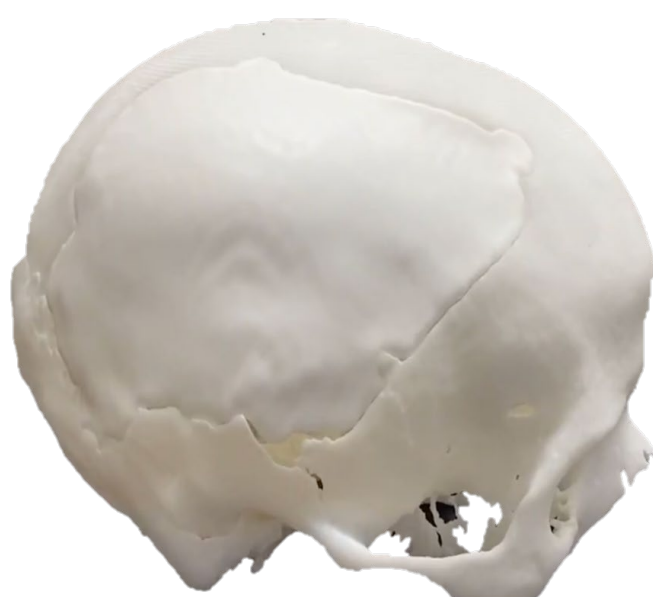
Figure 2: 3D Printed Cranial Implant designed by SHG AI Model
