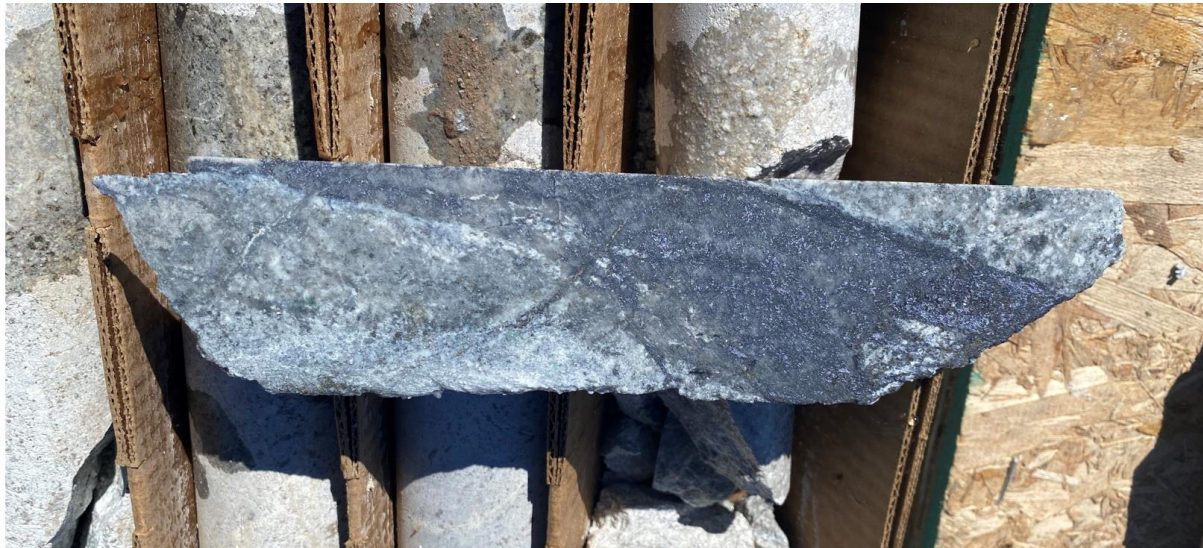
Figure 3: Strong quartz-pyrite-molybdenite veining in drill core from WD22-01 (768.67m downhole)
