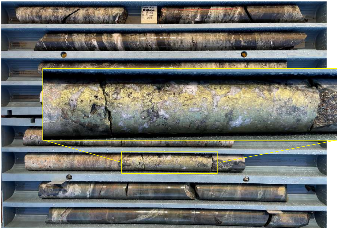
v. Banded magnetite-pyroxene-brown garnet skarn in volcanoclastic sandstone @ 845.9-852.9m, with insert including massive chalcopyrite
