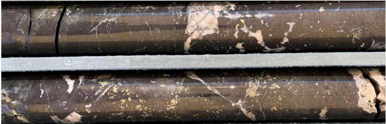
iv. Massive magnetite with disseminations of chalcopyrite and pyrite @ 824.5-825.6m
