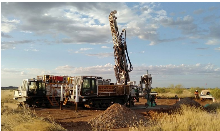
Figure 1 – RC rig drilling collar at hole DDH02
