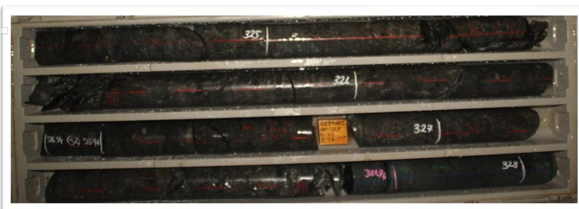
Figure 4 - Diamond Hole NRDD002 (Dry and wet) – Tray #92 - Disseminated sulphide (pentlandite 2%) from 323.3m to 327.4m
