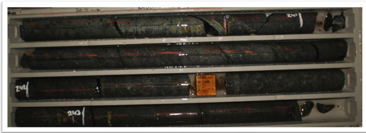
Figure 5 – Diamond Hole NRDD001 (Dry and wet) – Disseminated sulphide (pentlandite 1%) from 242m - 243m
