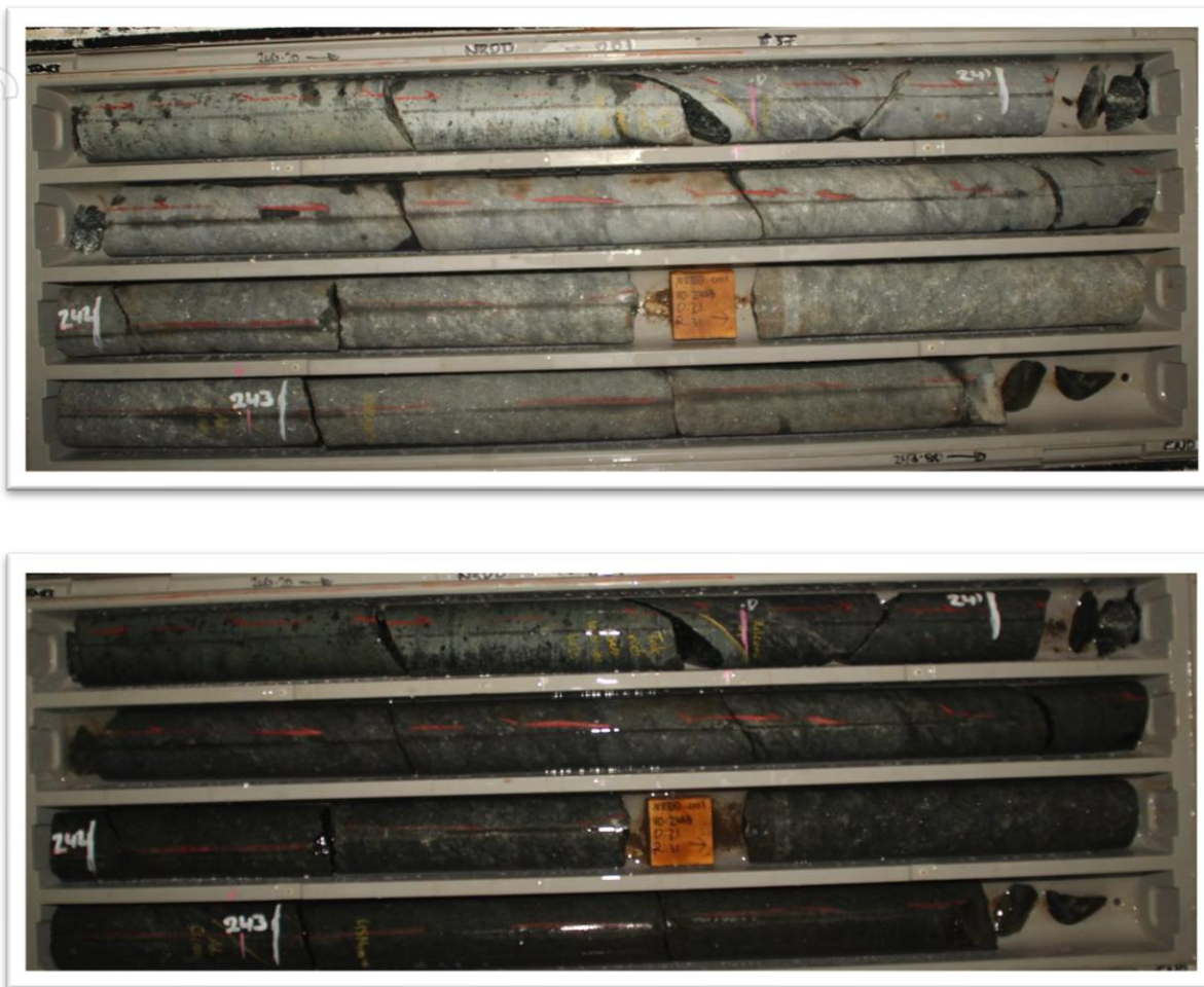
Figure 5 – Diamond Hole NRDD001 (Dry and wet) – Disseminated sulphide (pentlandite 1%) from 242m – 243m
