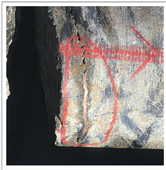
Figure 1 – Diamond Hole -NRDD002 - Native copper – 51.67m
