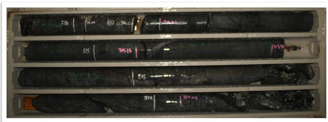
Figure 2 – Diamond Hole NRDD002 (Dry and wet) - Semi massive sulphide (pentlandite (5%) and chalcopyrite (5%)) from 315.57m to 317.08m
