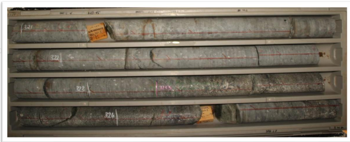
Figure 2 – Diamond Hole NRDD002 (Dry and wet) - Semi massive sulphide (pentlandite (5%) and chalcopyrite (5%)) from 315.57m to 317.08m
