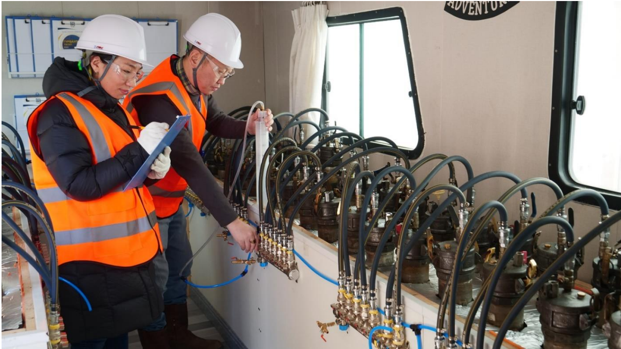
Figure 1 – Gas desorption monitoring at TMK Energy's on-site laboratory
